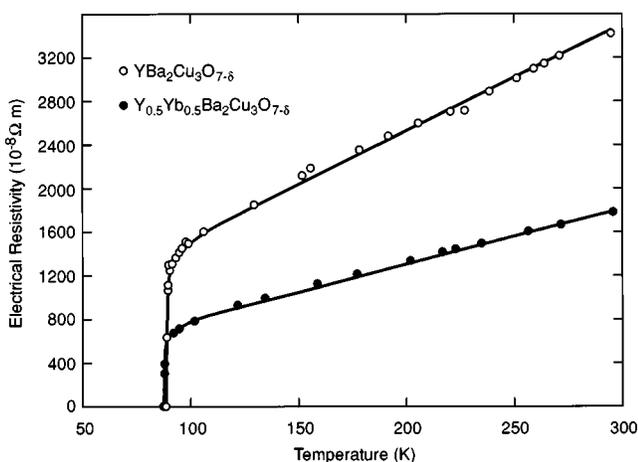
FIG. 1. Electrical resistivity data for Y123 and YYb123. Four probe dc measurements were obtained after the thermal-conductivity data had been obtained.
