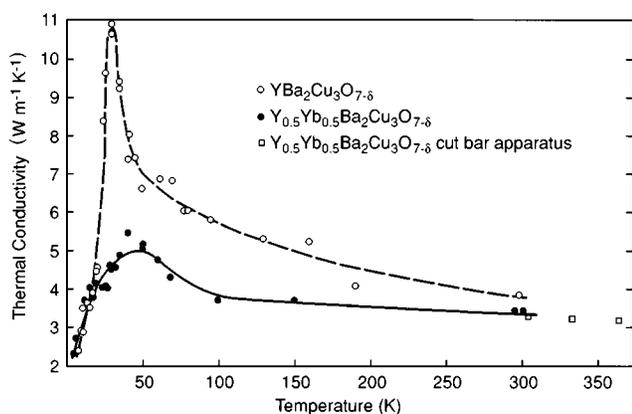
FIG. 3. Thermal-conductivity data for polycrystalline Y123 and  $\text{Y}_{0.5}\text{Yb}_{0.5}\text{Ba}_2\text{Cu}_3\text{O}_{7-\delta}$ . The lower-temperature measurements were made in a guarded longitudinal heat-flow apparatus (Ref. 9) and data obtained in an ambient temperature cut-bar apparatus are included to demonstrate accuracy and batch-to-batch variability.
