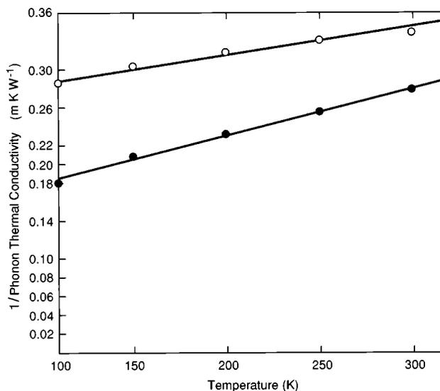
FIG. 4. Estimated phonon thermal-resistivity curves for Y123 and  $\text{Y}_{0.5}\text{Yb}_{0.5}\text{Ba}_2\text{Cu}_3\text{O}_{7-\delta}$ . The Sommerfeld-Lorenz number and the data shown in Fig. 1 were used to correct for electronic transport.
