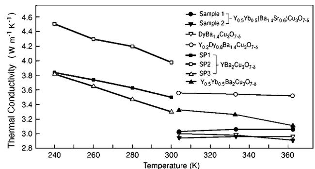
FIG. 2. Ambient temperature thermal-conductivity data for five partially substituted Y123 samples. The data for three Y123 samples are from Ref. 11.
