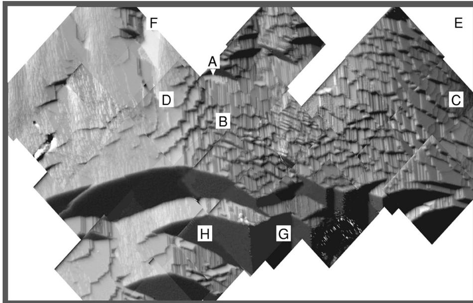
FIG. 2. A large-scale STM image ( $8000 \text{ \AA} \times 5000 \text{ \AA}$ , 2.0 V, 50 pA, a tiling of many small images) of the heteroepitaxial germanium layer grown on Si(103), showing the hill-and-valley morphology of the completely faceted germanium surface. Facets marked A through H are Ge(105), (103), (216),  $(2\bar{1}6)$ , (113),  $(1\bar{1}3)$ ,  $(15\bar{3}23)$ , and  $(15\bar{3}2\bar{3})$ , respectively. Note that this figure is rotated clockwise by  $45^\circ$  to save space.
