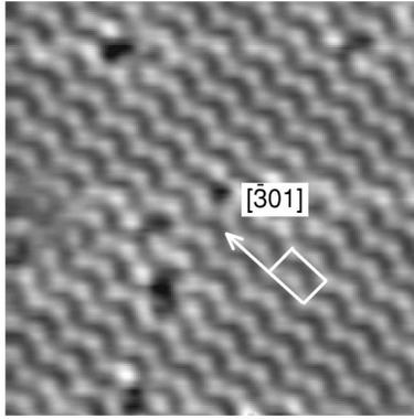
FIG. 4. A high-resolution STM image of the Si(103)  $1 \times 1$ -In surface,  $77 \text{ \AA} \times 77 \text{ \AA}$ ,  $-1.5 \text{ V}$ ,  $1.5 \text{ nA}$ .
