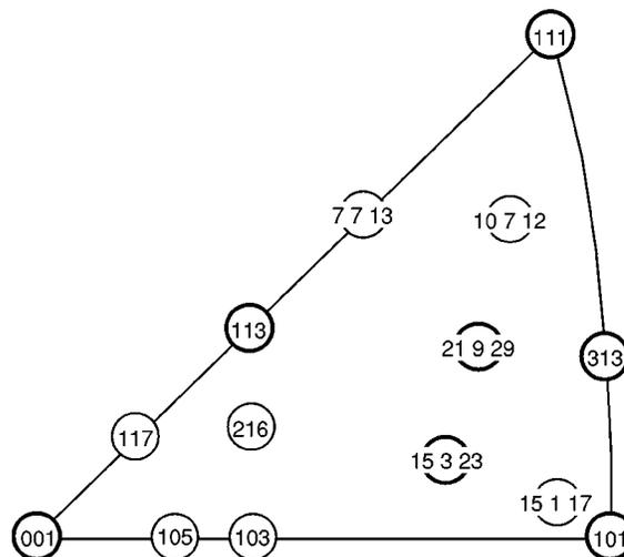
FIG. 1. Unit stereographic triangle, showing the seven major stable (thick circles) and seven minor stable surfaces (thin circles) of germanium determined recently (Refs. 17-23).
