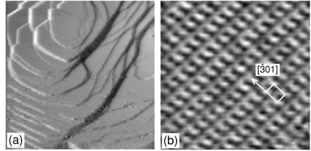
FIG. 5. STM images of the Ge(103)  $1 \times 1$ -In surface structure of the heteroepitaxial germanium layer on Si(103). (a)  $2460 \text{ \AA} \times 2460 \text{ \AA}$ ,  $2.5 \text{ V}$ ,  $20 \text{ pA}$ . (b)  $77 \text{ \AA} \times 77 \text{ \AA}$ ,  $-1.2 \text{ V}$ ,  $200 \text{ pA}$ .
