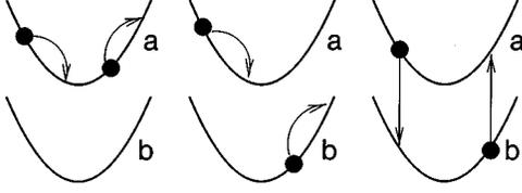
FIG. 2. Change of electron states in processes corresponding to parts of the Coulomb interaction (from left to right): band gap renormalization  $V_q^{aaaa}$ , excitonic enhancement  $V_q^{abba}$ , and depolarization  $V_q^{abab}$ .
