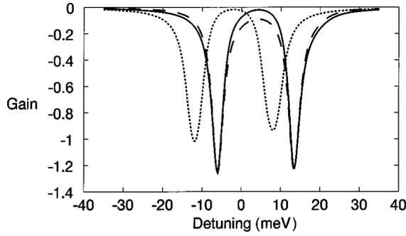
FIG. 3. Gain spectrum for a small subband dispersion (corresponding to a GaAs QW) as a function of detuning  $\Delta$  with no injection into subbands  $a$  and  $a'$  with Coulomb terms and Fano interference (solid curve), with Coulomb terms without Fano interference (dashed curve), and without Coulomb terms with Fano interference (dotted curve).
