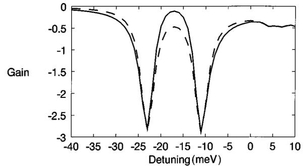
FIG. 6. Gain spectrum for interband transitions (corresponding to a GaAs QW) as a function of detuning  $\Delta$  with no injection into subbands  $a$  and  $a'$  with Coulomb terms and Fano interference (solid curve) and with Coulomb terms without Fano interference (dotted curve).
