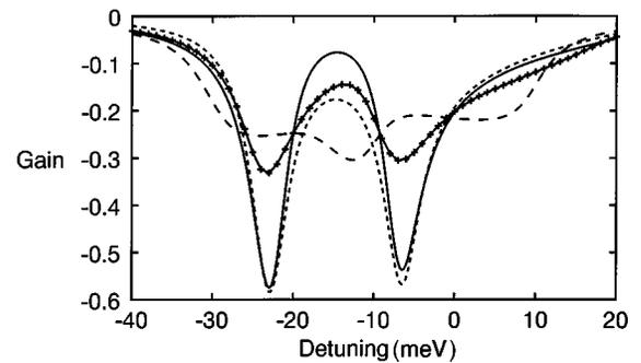
FIG. 5. Gain spectrum for a large subband dispersion (corresponding to an InAs QW) as a function of detuning  $\Delta$  with no injection into subbands  $a$  and  $a'$  with Coulomb terms and Fano interference (solid curve), with Coulomb terms without Fano interference (dotted curve), and without Coulomb terms with Fano interference (dashed curve). The curve with crosses corresponds to injection into subbands  $a$  and  $a'$  with the account of all terms.
