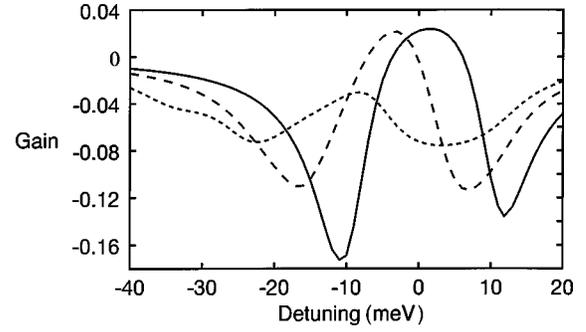
FIG. 4. Gain spectrum as a function of detuning  $\Delta$  with the injection into subbands  $a$  and  $a'$  for  $m_a = 0.042$  (corresponding to a GaAs QW), solid curve; for  $m_a = 0.033$ , dashed curve; and  $m_a = 0.028$  (corresponding to an InAs QW), dotted curve.
