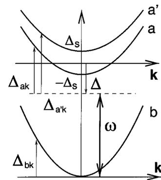
FIG. 1. Scheme of the momentum states of subbands  $a$  and  $a'$  coupled by a laser field with the frequency  $\omega$  to subband  $b$ . Here  $\Delta_{a\mathbf{k}}$ ,  $\Delta_{a'\mathbf{k}}$ , and  $\Delta_{b\mathbf{k}}$  are the detunings of the states from the field and  $\Delta = -(\Delta_{a0} + \Delta_{a'0})/2$ .
