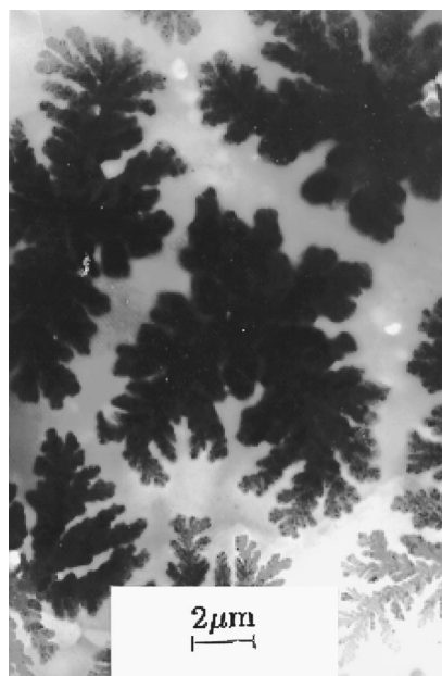
FIG. 8. Bright field transmission electron micrograph of the PPO film implanted at a fluence of 5 \times 10^{16} ions/cm 2 showing the growth of larger fractal patterns containing carbonaceous clusters.
