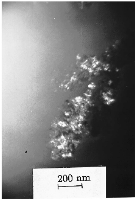
FIG. 10. Dark field transmission electron micrograph of the PPO film implanted at a fluence of 5 \times 10^{16} ions/cm 2 .
