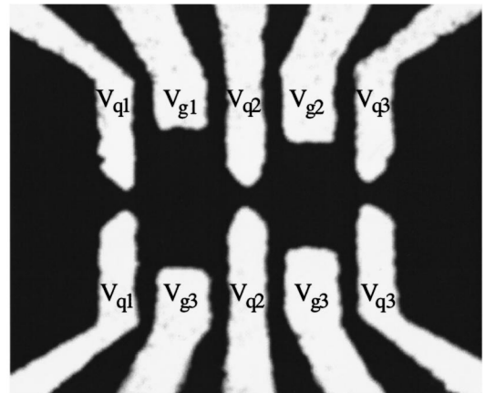
FIG. 1. Scanning electron micrograph of an asymmetric double quantum dot device. Light regions are the metal surface gates; dark regions are the wafer surface. The gate wiring is indicated.
