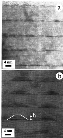
FIG. 1. HREM pictures showing a  $\langle 2\text{-}1\text{-}10 \rangle$  cross section of stacked layers of GaN dots. (a) Small dots about 2.3 nm high. Unburied dots protected by the glue are visible in the sample surface. (b) Large dots about 4.1 nm high grown with a ripening step under vacuum between successive layers.
