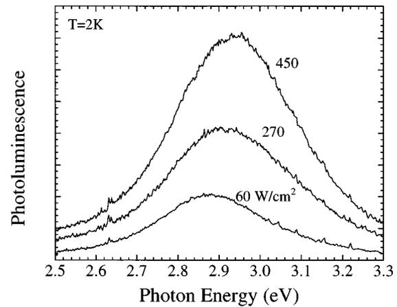
FIG. 4. Influence of the excitation density on the photoluminescence energy of large dots.
