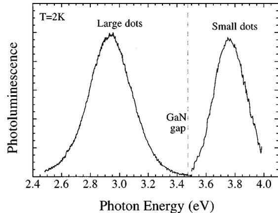
FIG. 2. Photoluminescence spectra of GaN quantum dots at  $T=2$  K. Note the large redshift observed for the 4.1-nm-high dots with respect to the small ones.
