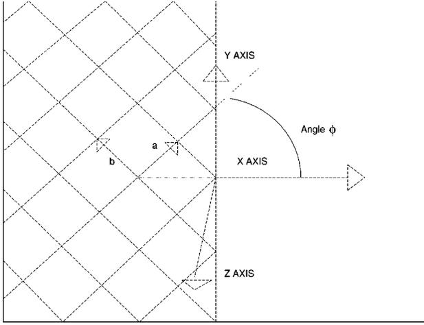
FIG. 1. The orientation of the crystal planes to the surface and the coordinate axes.  $\hat{a}$  and  $\hat{b}$  are unit vectors along the crystal axes.
