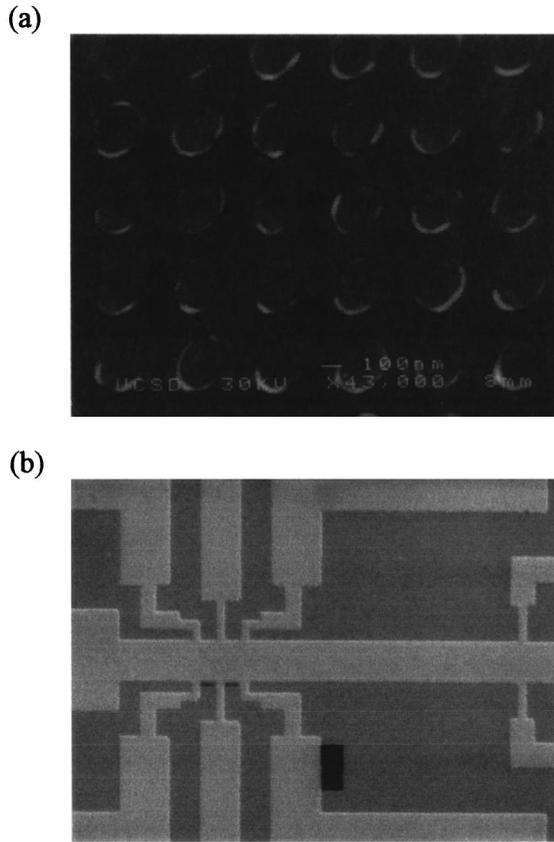
FIG. 1. (a) SEM image of a square array of Ni magnetic dots fabricated by  $e$ -beam lithography on a Si substrate. The lattice constant is  $d=400\pm 10$  nm and the Ni dots have a diameter  $c=200\pm 20$  nm. (b) Micrograph of the  $40\ \mu\text{m}$  width Nb bridge defined by optical lithography and RIE in the array region.
