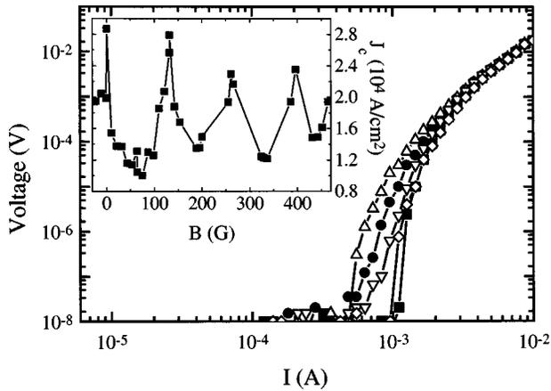
FIG. 4.  $I$ - $V$  curves as a function of field at  $T=7.7$  K for the  $100 \pm 10$  nm thick Nb film on top of the square array of Ni dots. The curves are shown for the following fields: 0 G (■), 10 G (●), 64 G (△), 110 G (▽), 132 G (◇). Inset shows the critical current extracted from the  $I$ - $V$  curves with a  $5 \times 10^{-3}$  V/m criteria.
