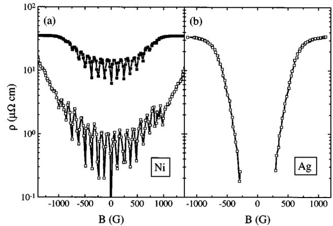
FIG. 2. Field dependence of the resistivity of a  $100\pm 5$  nm thick Nb bridge on top of a square array of Ni or Ag dots with a lattice spacing of  $d=400\pm 10$  nm. The applied current density is  $J=2.5\times 10^2$  A/cm<sup>2</sup>. (a) Two curves with temperatures of  $T=8.1$  K (■) and  $T=7.9$  K (□) are presented for the Ni. (b) For comparison, the curve presented for Ag was measured at  $T=7.9$  K.
