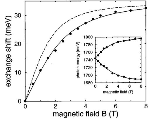
FIG. 1. Exchange shift of sample 1 at  $T = 1.6$  K. The experimental results are indicated by full circles. The full (dashed) line represents the theoretical calculations including (ignoring) alloy clustering effects. (The Zeeman splitting of the barrier transition for this sample is shown in the inset together with a fit to a modified Brillouin function corresponding to “random”  $\text{Cd}_{0.906}\text{Mn}_{0.094}\text{Te}$  bulk material.)
