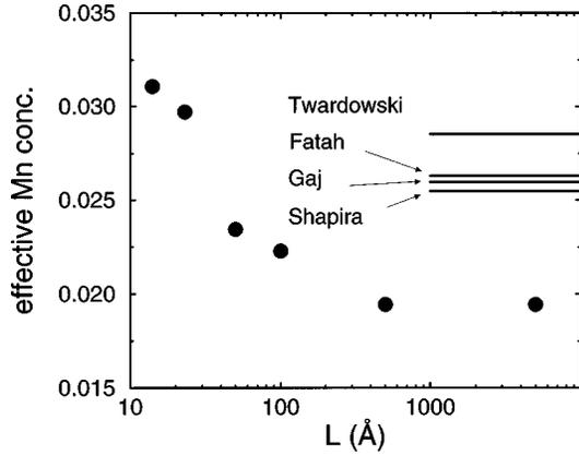
FIG. 4. Effective Mn ion concentration in  $\text{Zn}_{0.96}\text{Mn}_{0.04}\text{Se}$  layers of varying width  $L$ . The data points (full circles) were obtained by Heimbrodt *et al.* (Ref. 25). The bulk values (horizontal lines) were taken from Twardowski *et al.* (Ref. 27), Fatah *et al.* (Ref. 3), Gaj *et al.* (Ref. 2) and Shapira (Ref. 8).
