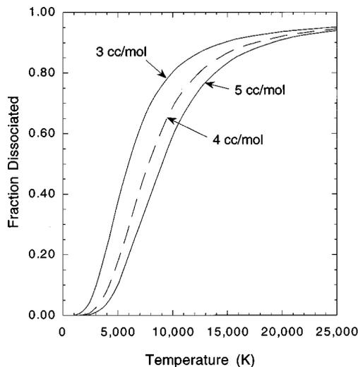
FIG. 7. Calculated fractions of  $D_2$  molecules dissociated vs temperature at several volumes.
