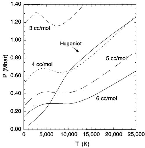
FIG. 6. Calculated isochores and the liquid deuterium Hugoniot plotted as pressure vs temperature.
