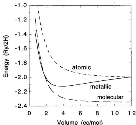
FIG. 2. Energy vs volume/(2H atoms) for lattices of molecular hydrogen (lower curve), metallic (middle curve), and atomic hydrogen (upper curve).
