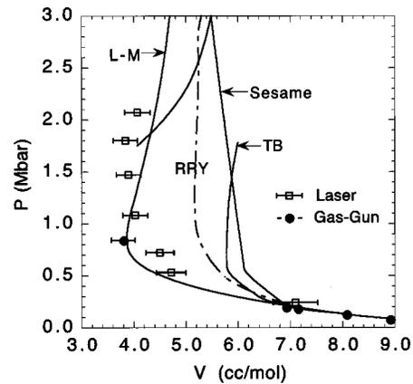
FIG. 5. Experimental shock data for deuterium with calculations from several models: linear-mixing (Fig. 3), RRY (Ref. 13), Sesame (Ref. 31), and tight-binding (TB) (Ref. 30).
