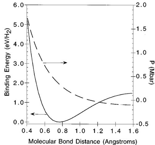
FIG. 11. LDA calculation of the total energy and pressure of an hcp lattice of hydrogen molecules at 0 K (Ref. 33) as the intramolecular bond distance is varied at a constant volume of 4 cc/mol.
