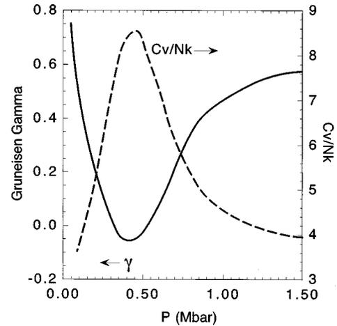
FIG. 8. Gruneisen Gamma ( $\gamma$ ) and reduced heat capacity ( $C_V/Nk$ ) vs pressure calculated along the Hugoniot.
