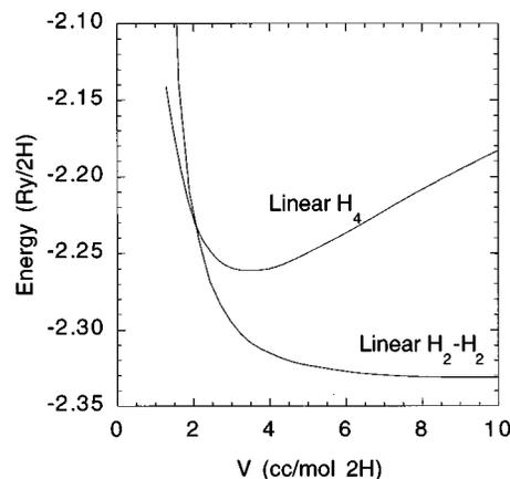
FIG. 1. Configuration interaction calculation of the total energy for  $H_2$ - $H_2$  and linear  $H_4$  taken from the tables of Bender and Schaefer (Ref. 16). The data has been plotted in terms of the volume approximated as the sphere occupied by an inner atom of the equidistant  $H_4$  chain for equal linear lengths of  $H_4$  and  $H_2$ - $H_2$ .
