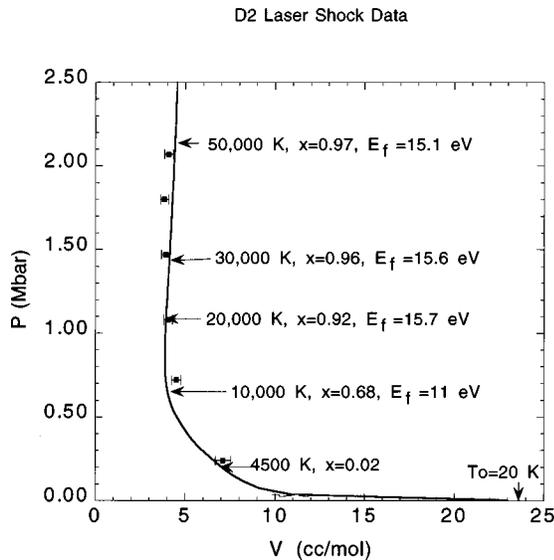
FIG. 4. Experimental laser shock data for deuterium with calculated, Hugoniot, shock temperatures, dissociated fractions ( $x$ ), and Fermi energies ( $E_f$ ) at selected pressures.
