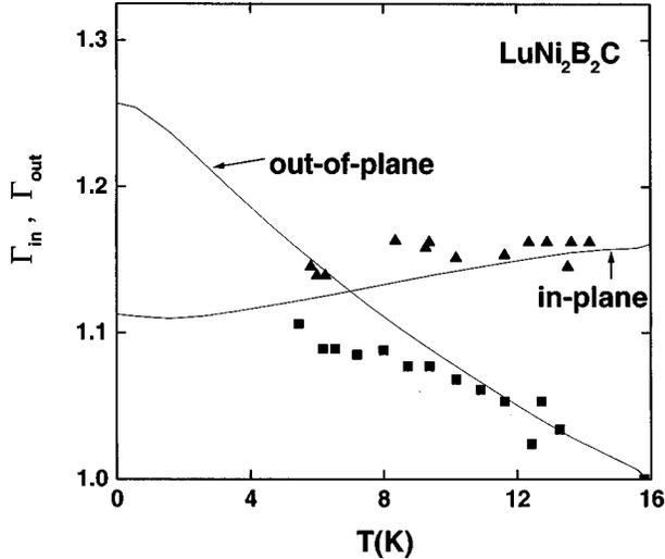
FIG. 5. The out-of-plane and the in-plane anisotropies are shown as a function of temperature. The black squares are the experimental data taken from (Ref. 12).
