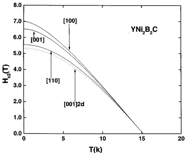
FIG. 2. The upper critical fields for different field direction for  $m_c/m_b=1$  are shown as a function of temperature. The temperature dependences are similar to those observed in  $\text{YNi}_2\text{B}_2\text{C}$  (Ref. 17).
