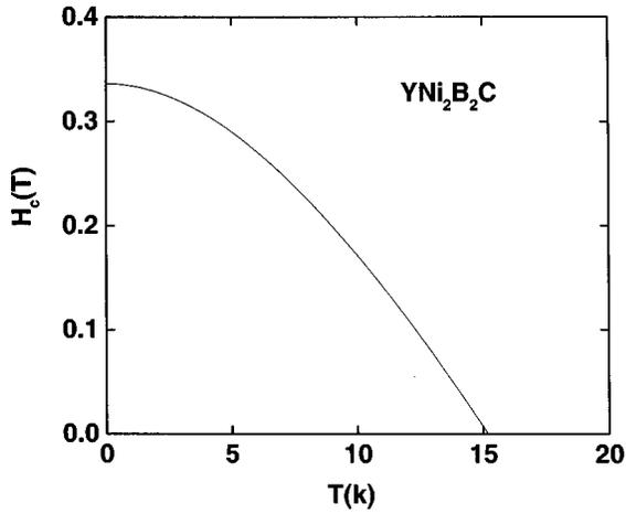
FIG. 1. The thermodynamically critical field of a  $d$ -wave superconductor is shown as a function of  $T$ . Here we adjust the slope of  $H_c(T)$  at  $T=T_c$  with the experimental value (Ref. 17).
