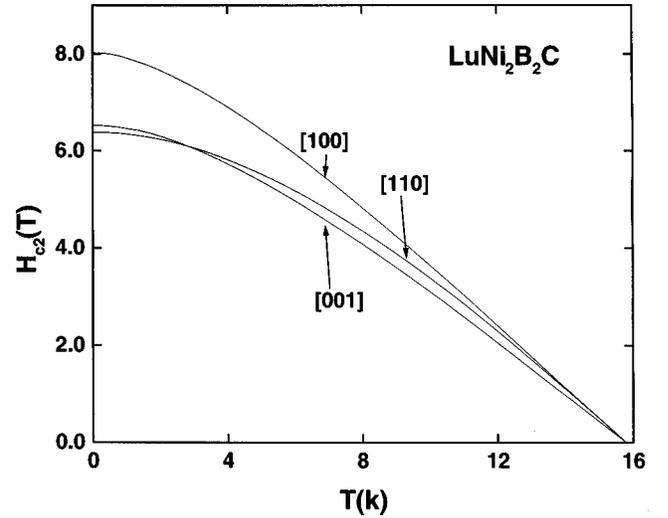
FIG. 3. The same as in Fig. 2 but for  $m_c/m_a=1.35$ . The temperature dependences are compared with the experimental data for  $\text{LuNi}_2\text{B}_2\text{C}$  (Ref. 12).
