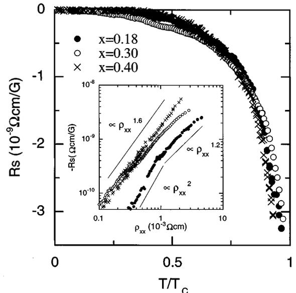
FIG. 3. Temperature dependence of the anomalous Hall coefficient  $R_s$  for  $x=0.18$ ,  $0.30$ , and  $0.40$ . The inset shows  $-R_s$  as a function of longitudinal resistivity  $\rho_{xx}$ .
