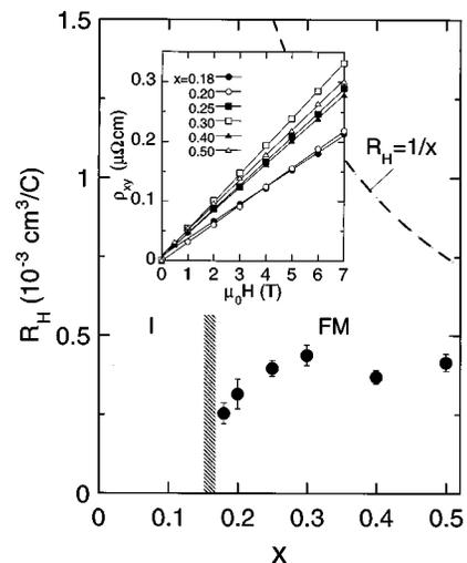
FIG. 1. Ordinary Hall coefficient  $R_H$  of  $\text{La}_{1-x}\text{Sr}_x\text{MnO}_3$  crystals with  $x = 0.18-0.50$  at 4.2 K. The nominal carrier number ( $n$ ) calculated from  $R_H$  using  $R_H = 1/en$  is about  $1.5-2.0 \times 10^{22} \text{ cm}^{-3}$  or  $\approx 1$  hole/Mn site. The Hall resistivity  $\rho_{xy}$  at 4.2 K as a function of applied field is shown in the inset. I and FM denote insulating and ferromagnetic metallic states, respectively.
