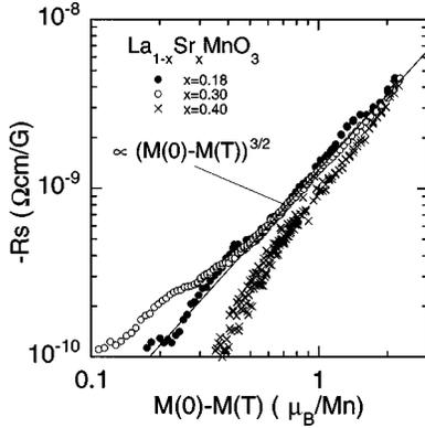
FIG. 4.  $-R_s$  is plotted for  $x=0.18, 0.30$ , and  $0.40$  with the change of magnetization  $[M(0) - M(T)]$ , where  $M(0)$  denotes the saturated magnetization at zero temperature. A solid line represents the empirical relation  $R_s = -1.3 \times 10^{-9} [M(0) - M(T)]^{3/2}$ ,  $R_s$  and  $M$  being in units of  $\Omega \text{ cm/G}$  and  $\mu_B/\text{Mn}$  site, respectively.
