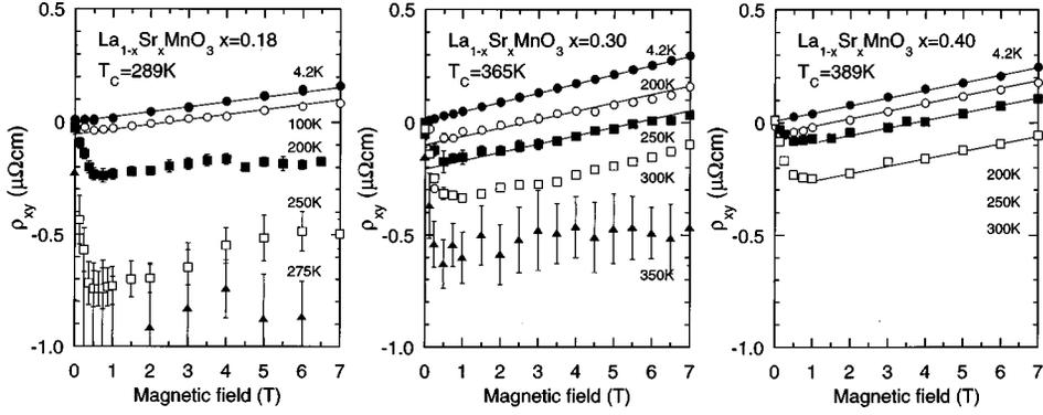
FIG. 2. The Hall resistivity  $\rho_{xy}$  as a function of applied field at various temperatures for  $x=0.18$  (left panel),  $0.30$  (middle panel), and  $0.40$  (right panel).
