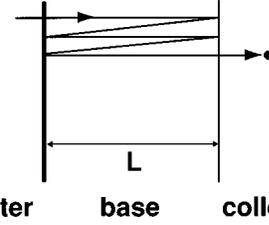
FIG. 7. This figure shows schematically that electrons with energy close to  $eV_b = 0.8$  eV have a small transmission coefficient  $T$  at the base/collector interface and that their path length is long owing to the multiple reflection in the base with thickness  $L$ .
