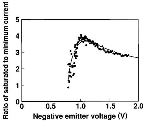
FIG. 2. Dependence of the ratio of saturated to minimum collector current (MR ratio) on the emitter voltage in type A measured at 77 K. The solid curve is a plot of Eq. (8) with the approximation for  $I_e(V)$  of Eq. (10), where three parameters,  $l_{\uparrow}$ ,  $l_{\downarrow}$ , and  $l_{sf}$ , are set at 5.3, 2.9, and 106 nm, respectively.
