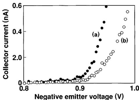
FIG. 3. Voltage dependence of the collector current below 1 V. Curves (a) and (b) are for the saturated and minimum current, respectively.
