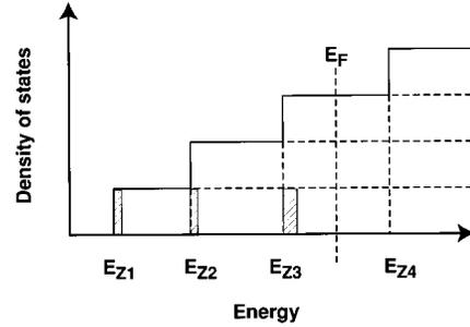
FIG. 9. Schematic density of states in a two-dimensional system. Only electrons in the hatched areas take part in tunneling due to the strong forward focusing effect of tunneling electrons.
