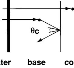
FIG. 6. This figure shows schematically that most electrons scattered outside  $\theta_c$  in the base cannot flow into the collector. These electrons decay in the base as a result of inelastic scattering and flow out as a base current.
