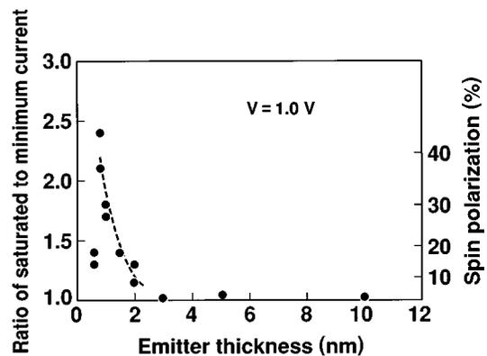
FIG. 5. Dependence of the MR ratio at 1 V on the thickness of Fe in the emitter. The values of spin polarization of tunneling electrons estimated by using Eqs. (14) and (15) are also plotted on the right-hand side ordinate. A broken curve in the figure is a guide to the eye.
