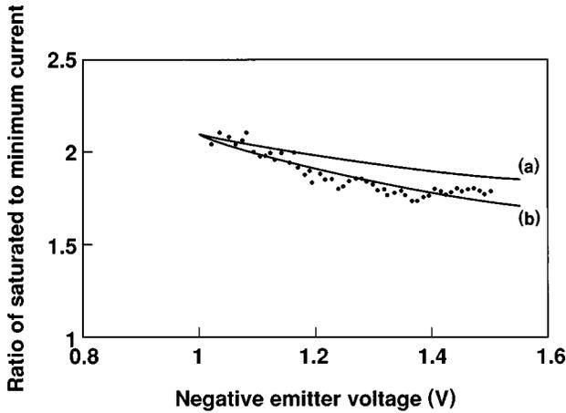
FIG. 8. The voltage dependence of the MR ratio observed in type *B*. Thickness of Fe in the emitter is 0.8 nm. Curve (a) is a plot of Eq. (14) with  $P=0.37$ . In curve (b),  $P$  changes linearly with voltage from 0.37 at 1 V to 0.25 at 1.5 V.
