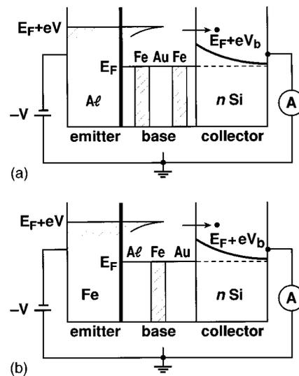
FIG. 1. (a) Schematic energy diagram of the three-terminal structure of type A. Hot electrons are injected into the base by applying a voltage *V* to the emitter. Hot electron current that flows into the collector is detected as a collector current. *eV<sub>b</sub>* is the Schottky barrier height. (b) Schematic energy diagram of the three-terminal structure of type B. Spin-polarized electrons are injected from an Fe emitter into an Al/Fe/Au base.
