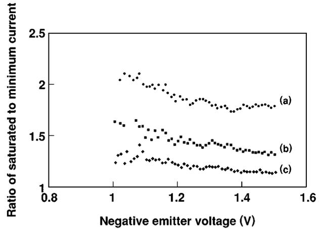
FIG. 4. Dependence of the MR ratio on the emitter voltage in type B measured at 77 K. Thickness of Fe in the emitter is (a) 0.8 nm, (b) 1 nm, and (c) 2 nm, respectively.
