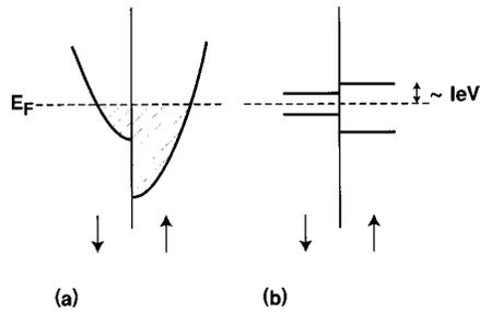
FIG. 10. (a) Schematic density of states of  $s$  bands in Fe. (b) Quantized energy levels of  $s$  electrons in an ultrathin Fe film.
