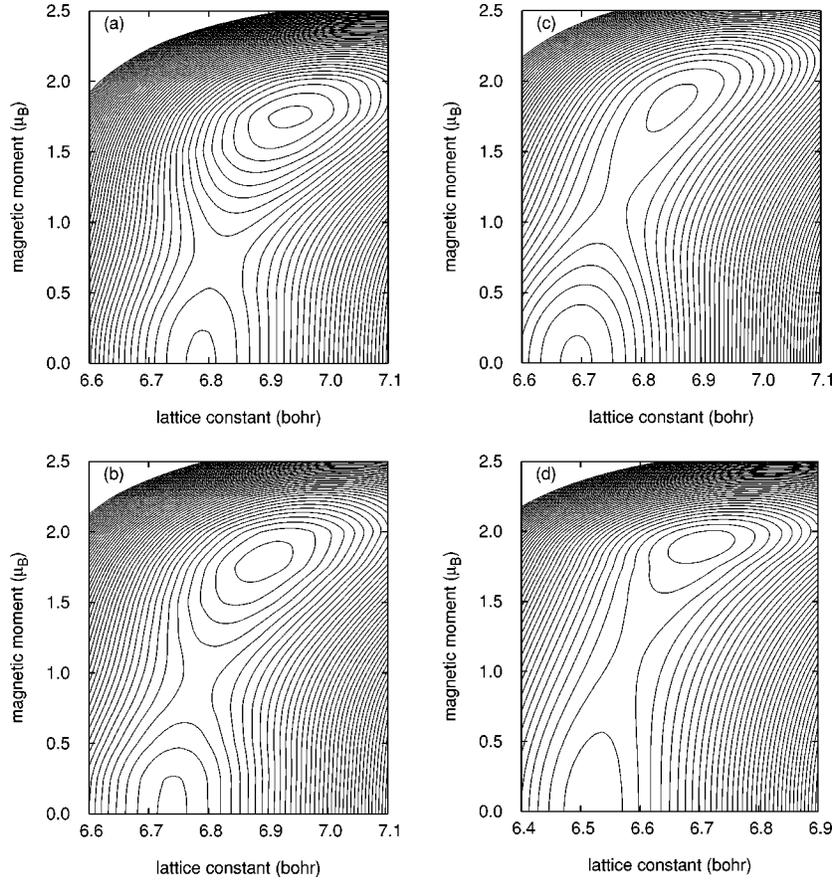
FIG. 2. Contour plots of  $E_{\text{tot}}(a, m)$  for (a)  $\text{Fe}_{0.70}\text{Pt}_{0.30}$ , (b)  $\text{Fe}_{0.75}\text{Pt}_{0.25}$ , (c)  $\text{Fe}_{0.80}\text{Pt}_{0.20}$ , and (d)  $\text{Fe}_{0.70}\text{Ni}_{0.30}$ . The energy difference between neighboring isolines is 0.5 mRyd.
