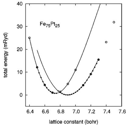
FIG. 3. Total energy  $E_{\text{tot}}(a)$  of high-moment and zero-moment solutions for  $\text{Fe}_{0.75}\text{Pt}_{0.25}$ . The different solutions have been found by changing the lattice constant inwards (filled circles) or outwards (big open circles), respectively. The absolute minimum of the energy has been set to zero, and the lines result from polynomial interpolation.
