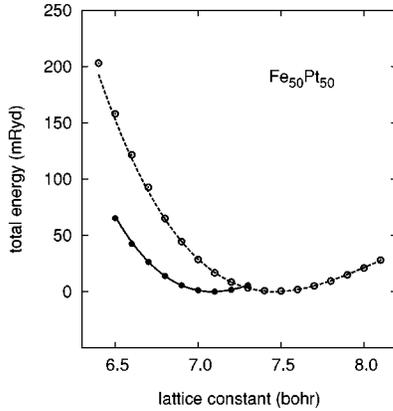
FIG. 1. Nonrelativistic (open circles, dashed line) and scalar relativistic (filled circles, full line) total energy  $E_{\text{tot}}(a)$  for  $\text{Fe}_{0.50}\text{Pt}_{0.50}$  as a function of the lattice constant  $a$ . The minima of both curves have been set to zero energy, and the lines are due to a polynomial interpolation of the nonmagnetic values.
