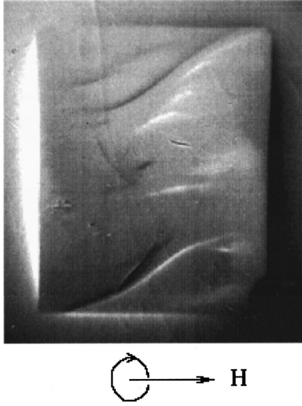
FIG. 11. Splitting of the Meissner hole images. The field was decreased from 970 to 490 G after rotation by 360^\circ . T = 40 K.
