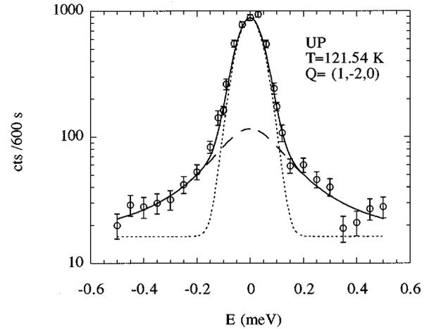
FIG. 4. Inelastic scan taken at  $Q=(1\bar{2}0)$  in the paramagnetic phase of UP. A clear quasielastic peak is seen in addition to the incoherent (elastic resolution limited) scattering. Counting time was  $600$  s per point.
