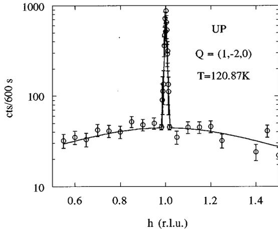
FIG. 1. An example of the two-component line shape (in wave vector) at the  $(1\bar{2}0)$  position seen in the vicinity of  $T_N$ . Data is the difference of the elastic scattering at 120.87 K and 200 K (background) taken with incident neutrons having  $k_i = 1.55 \text{ \AA}^{-1}$ .
