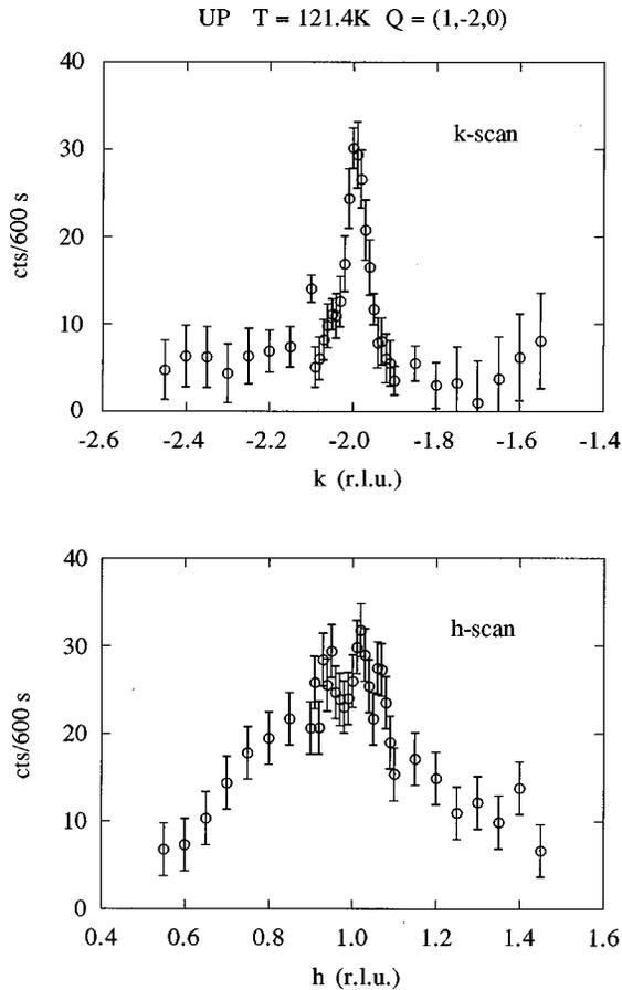
FIG. 3. The highly anisotropic line shape in wave-vector space at the  $(1\bar{2}0)$  position seen at  $T=121.4$  K (above  $T_N$ ) in UP. The direction  $h$  lies parallel, antiparallel to the low-temperature sublattice magnetization directions. The direction  $k$  lies in the scattering plane and is orthogonal to the direction  $h$ .
