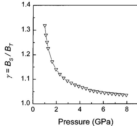
FIG. 3. Calculated ratio ( $\gamma$ ) of adiabatic ( $B_S$ ) and isothermal ( $B_T$ ) vs pressure.
