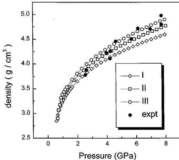
FIG. 1. The equation of state for solid krypton from 1 to 8 GPa.
