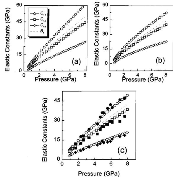
FIG. 2. Elastic constants for solid krypton calculated from several interatomic potentials (see text). (a) Lennard-Jones (potential I); (b) Bobetic (potential II), and (c) Buck (potential III). The solid symbols indicate experimental measurements from Ref. 1.
