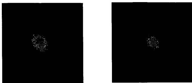
FIG. 3. ESDIAD patterns of F^- (left) and Cl^- (right) from CF_2Cl_2 -covered Ru(0001).
