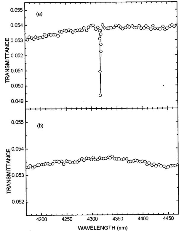
FIG. 2. FT-IR transmission spectra taken (a) before annealing and (b) after annealing. The absorption peak seen in (a) at the wavelength 4320 nm is the local vibration mode of  $V_{\text{In}}\text{H}_4$  complex.
