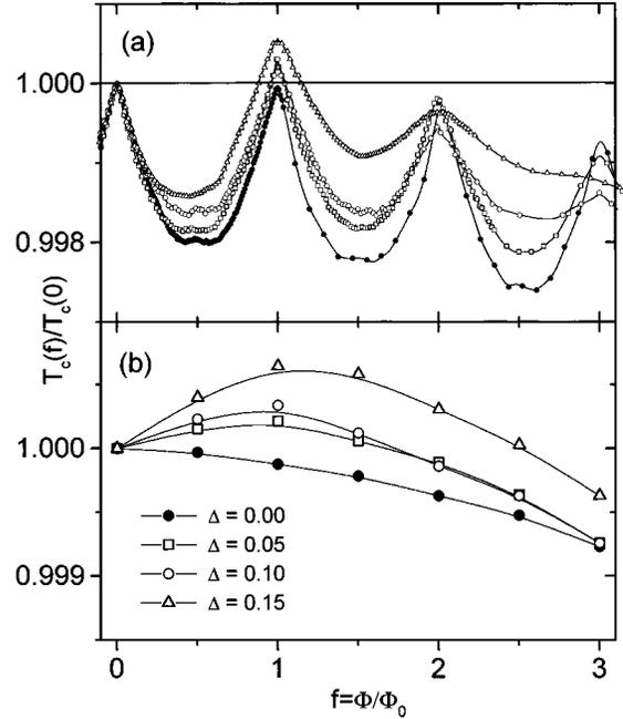
FIG. 2. (a) Normalized  $T_c$  vs  $\phi/\phi_0$ , for various disorder strengths. (b) Midpoints of each oscillation half period of the normalized  $T_c$  vs  $\phi/\phi_0$  shown in (a).
