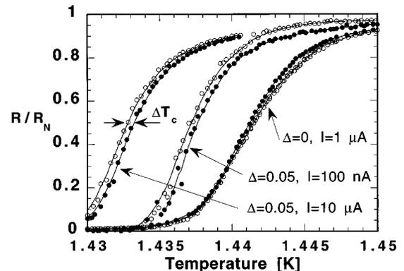
FIG. 3. Resistance vs temperature in the vicinity of the superconducting transition for disordered and regular networks at  $\phi/\phi_0=0$  (open symbols) and  $\phi/\phi_0=1$  (filled symbols).
