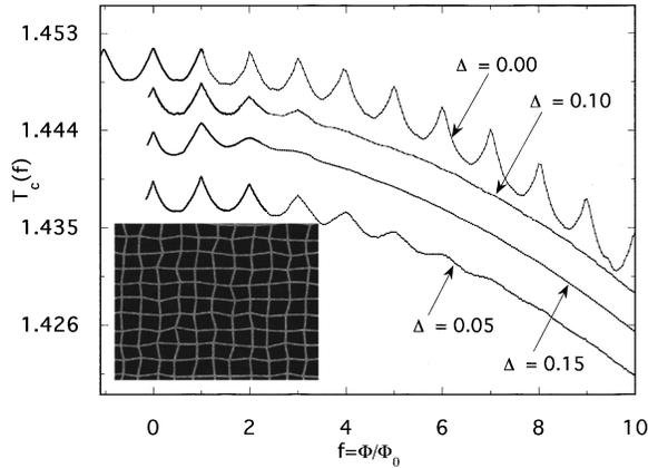
FIG. 1. Superconducting-normal phase boundary, defined by  $R/R_n=0.5$ , for networks with various disorder strengths  $\Delta$ . Note that  $\phi/\phi_0=1$  corresponds to  $H=5$  G. The vertical position of each curve is uncertain to 1%, due to variations in the thermometry after cycling to room temperature. Inset: SEM micrograph of a disordered array with  $\Delta=0.15$ .
