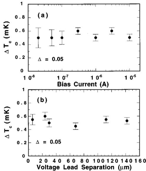
FIG. 4. (a) Critical temperature increase,  $\Delta T_c$ , for  $f=1$  relative to  $f=0$  [as illustrated in Fig. 3(a)] vs bias current for a network with  $\Delta=0.05$ . (b) The  $\Delta T_c$  vs voltage lead spacing, for the same network.
