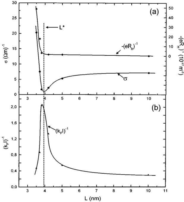
FIG. 1. (a) Normal state conductivity  $\sigma$  and conduction electron density  $n_e = -(eR_H)^{-1}$ ,  $R_H$  = Hall constant, and (b)  $(k_F l)^{-1}$  as obtained from  $\sigma$  and  $R_H$  within the Fermi gas model of granular Bi films as a function of Bi mean cluster size  $L$ . The solid lines through the data points are only guides to the eyes. The dashed vertical line indicates the critical cluster size  $L^*$  (see text).
