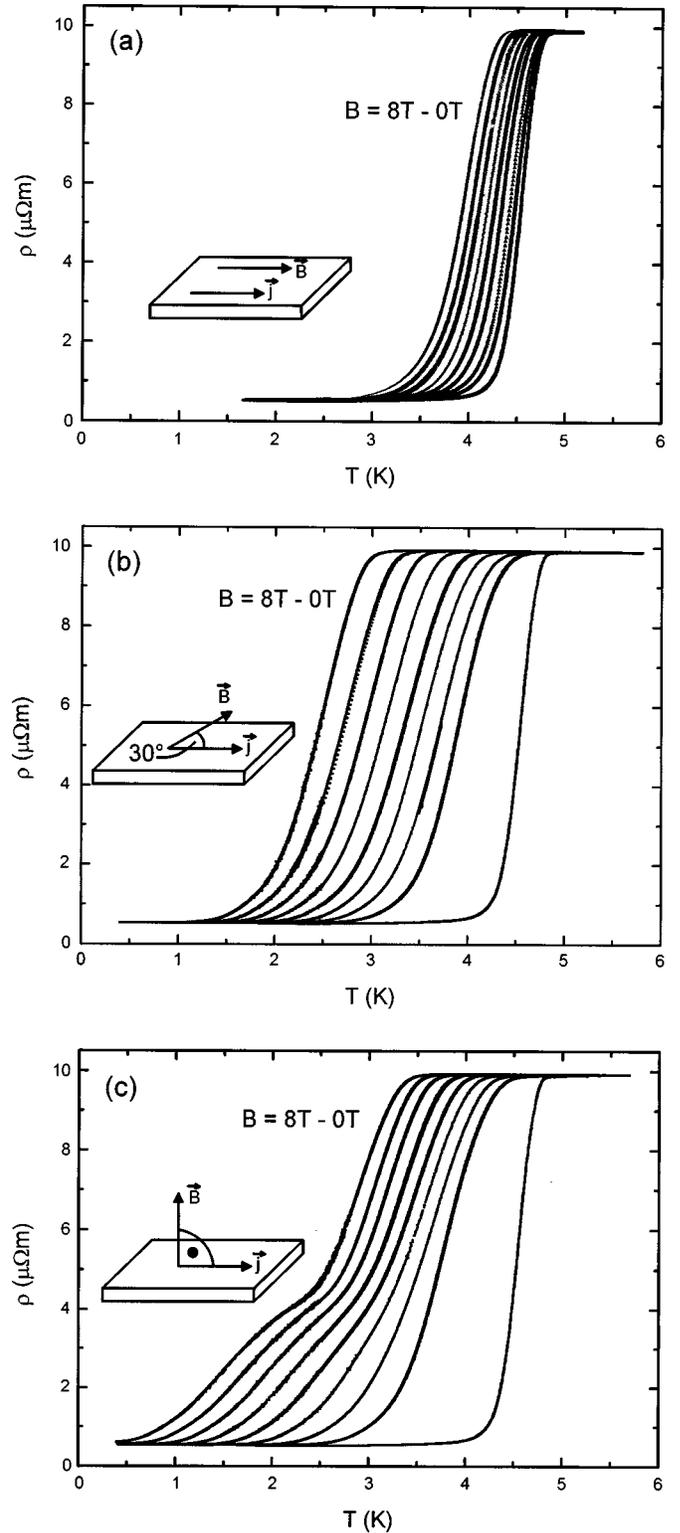
FIG. 2. Resistivity versus temperature for granular Bi film with  $L \approx 4.5$  nm as a function of external magnetic field  $B$ . The insets show the different directions of  $B$  relative to the current direction and the film plane, respectively.
