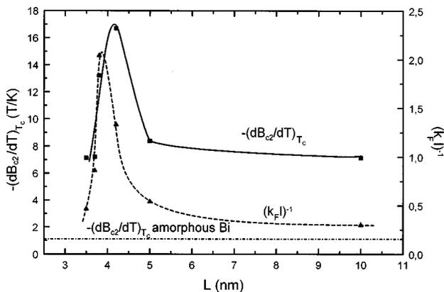
FIG. 4. Values of  $(dB_{c2}/dT)_{T_c}$  for granular Bi films as a function of Bi mean cluster size  $L$ . The solid line through the data points is a guide to the eyes. The dashed curve shows the  $(k_F l)^{-1}$  values from Fig. 1(b) for comparison. The  $(dB_{c2}/dT)_{T_c}$  value for amorphous Bi (from Ref. 8) is given by the dashed-dotted horizontal line.
