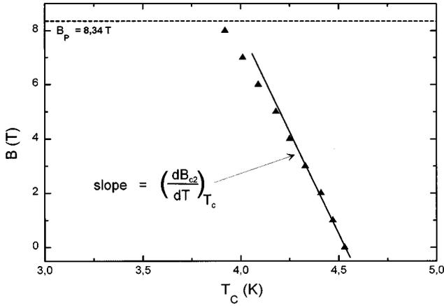
FIG. 3. Magnetic field dependence of superconducting transition temperature  $T_c$  of granular Bi film as obtained from Fig. 2(a). The solid line through the data points is a least-squares fit [straight line with slope  $(dB_{c2}/dT)_{T_c}$ ]. The horizontal dashed line gives the paramagnetic (Clogston) limit  $B_p$  (see text).
