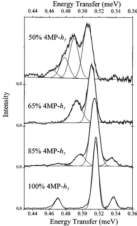
FIG. 1. Inelastic-neutron-scattering spectra of isotopic mixtures of the totally hydrogenated 4-methyl-pyridine molecule (4MP- $h_7$ ) and perdeuterated analogue (4MP- $d_7$ ). The temperature was 0.5 K for the isotopically pure sample (100% 4MP- $h_7$ ) and 1.8 K for the mixtures.
