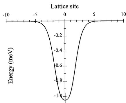
FIG. 4. Effective potential averaged over the internal oscillation for the breather interacting with an isolated deuterated molecule surrounded by hydrogenated molecules.
