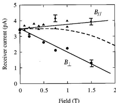
FIG. 3. Initial amplitude of THz emission as measured by receiver current [ $I_0$  in Eq. (1)] as a function of perpendicular (circles) and parallel (triangles) magnetic field. Continuous lines are guides to the eye, dashed line is a theoretical prediction for parallel field.
