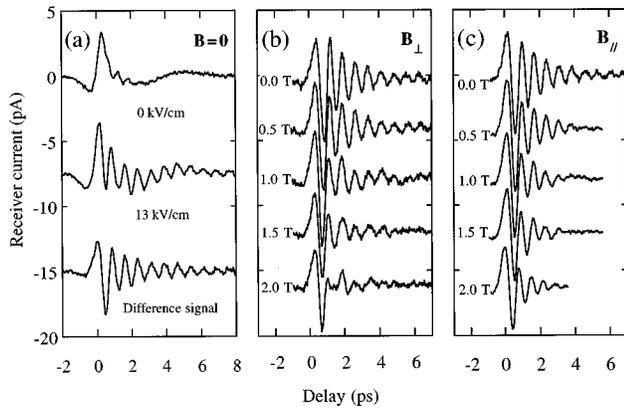
FIG. 1. Examples of THz emission spectra showing (a) the data subtraction procedure for background correction and (b), (c) the effect of perpendicular and parallel magnetic field on background corrected signals, respectively. The data has not been accurately corrected for propagation delay.
