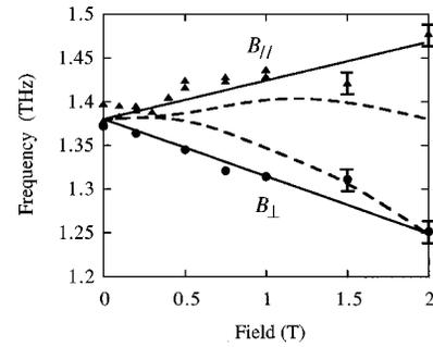
FIG. 4. Measured frequency of THz emission [ $f$  in Eq. (1)] as a function of perpendicular (circles) and parallel (triangles) magnetic field. Continuous lines are guides to the eye, dashed lines are theoretical predictions for parallel field (upper curve) and perpendicular field (lower curve).
