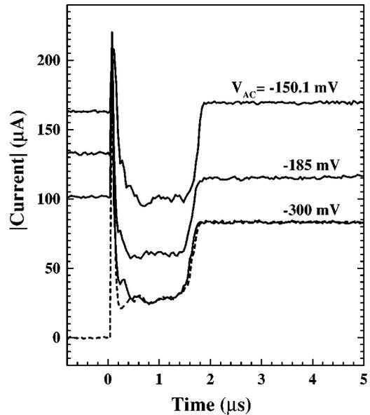
FIG. 5. Current response vs time for voltage pulse amplitudes of  $-150.1$ ,  $-185$ , and  $-300$  mV at an applied dc voltage of  $-0.7$  V (solid lines) and for  $-1.0$  V at an applied DC voltage of  $0$  V (dashed line) recorded at  $5$  K. The upper two solid lines have been shifted vertically in units of  $30 \mu\text{A}$  for clarity.
