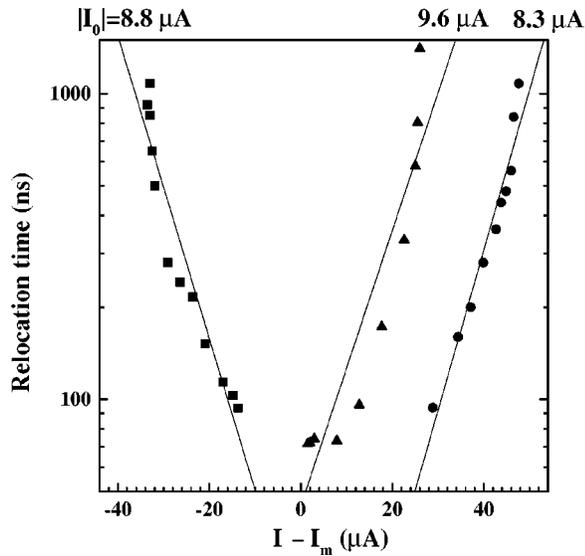
FIG. 4. Logarithm of the delay time vs current difference between final current value and the maximum or minimum current  $I_m$  of the initial branch. The squares correspond to the situation shown in Fig. 2(a), the triangles and circles to the situation in Fig. 3(a). The circles have been shifted horizontally by  $20 \mu\text{A}$ . The solid lines are linear fits to the data points.
