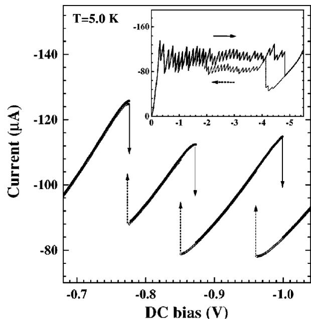
FIG. 1. Time-averaged  $I$ - $V$  characteristics at 5 K for two sweep directions, from 0 to  $-5.5$  V ( $\bullet$ ) and  $-5.5$  to 0 V ( $\diamond$ ). The complete sweep is shown for both directions in the inset.
