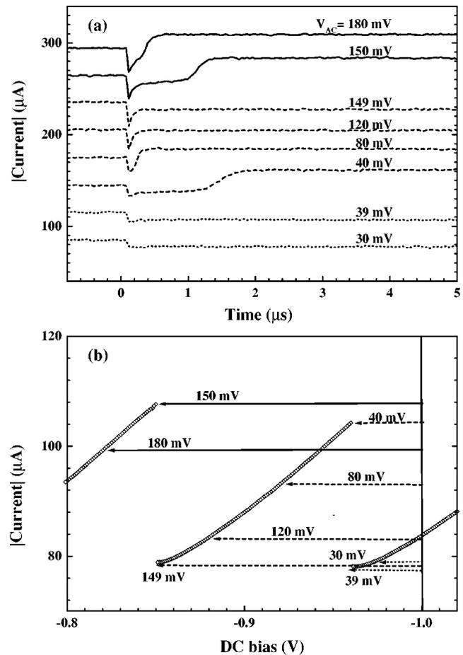
FIG. 3. (a) Current response vs time for different positive voltage pulse amplitudes at an applied dc voltage of  $-1.0$  V and 5 K. The curves have been shifted vertically in units of  $30 \mu\text{A}$  for clarity. (b) Section of the time-averaged  $I$ - $V$  characteristic indicating the total voltage applied during a voltage pulse.
