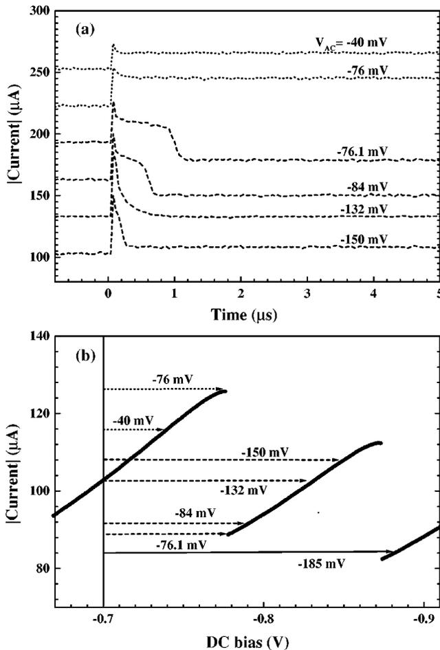
FIG. 2. (a) Current response vs time for different negative voltage pulse amplitudes at an applied dc voltage of  $-0.7$  V and 5 K. The curves have been shifted vertically in units of  $30 \mu\text{A}$  for clarity. (b) Section of the time-averaged  $I$ - $V$  characteristic indicating the total voltage applied during a voltage pulse.
