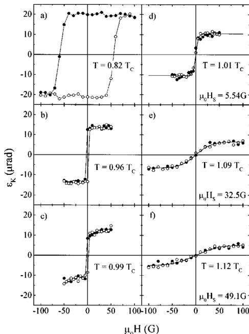
FIG. 2. Kerr ellipticity  $\varepsilon_K$  as a function of field  $H$  along  $[1\bar{1}0]$  for a system of ML stripes of width  $W=32$  (Fe coverage  $\Theta=0.8$  ML), for various temperatures  $T$  which are given in units of the Curie temperature  $T_C=179$  K of the sample. Full and open circles are for decreasing and increasing fields, respectively.
