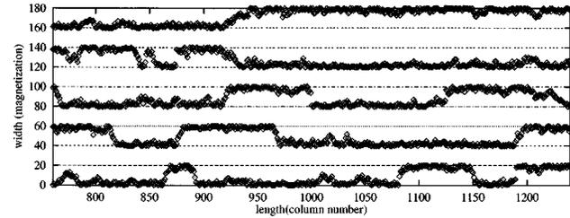
FIG. 5. Section ( $500 \times 180$ ) from a MC snapshot of a sample with  $W = 20$ , in a periodic model of noninteracting stripes. Alternating rows of width 20 represent either the Fe stripes or the bare tungsten stripes between. The Fe stripes are structured by a representation of their magnetization; see text.
