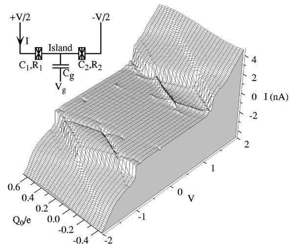
FIG. 1. Measured  $I(V, Q_0)$  surface for a SSS SET. Inset: bias schematic for the device.
