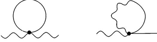
FIG. 8. Two diagrams that contribute to the renormalization of  $\Delta_1$ ,  $T\gamma$ , and  $\gamma$ . The full line corresponds to the correlator  $C^>$ , the full-wiggly line is the response function  $G^>$ , wiggly line is the  $\hat{\phi}$  field and the vertex is the  $S_1$  nonlinearity. The first diagram, is proportional to  $T$ , and is the graphical correction to  $\Delta_1$  and  $T\gamma$ , while the second one, survives even at zero temperature and renormalizes  $\gamma$ .
