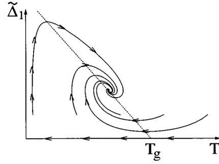
FIG. 5. Renormalization-group flow diagram (for  $2 < d = 2 + 0.3 < 3$ ) in the disorder  $\Delta_1$  temperature  $T$  plane, for a set of initial conditions with  $\bar{\Delta}_1(0) = 0.2$  and  $\bar{T}(0)$  ranging from 0.05 to 0.85, in increments of 0.2.
