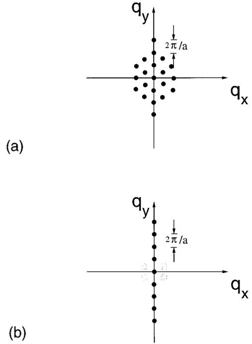
FIG. 2. (a) The static structure factor for the moving glass sketched in Fig. 1(a), with sharp peaks at all the reciprocal-lattice vectors of a triangular lattice. The static structure factor of the driven transverse smectic is shown in (b). Sharp peaks (dark spots) only appear along the  $q_y$  axis; some remnant of short-range local triangular lattice order can appear in the form of weak and diffuse peaks at finite  $q_x$  (light spots).
