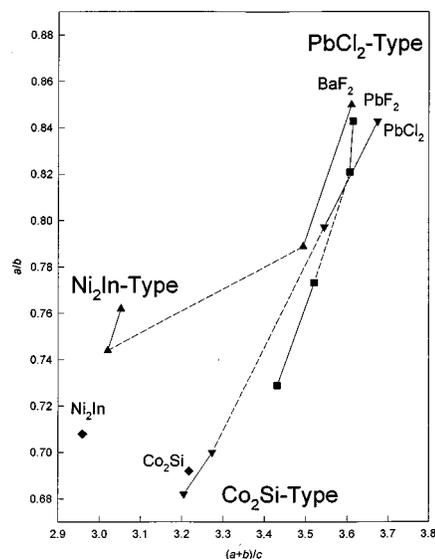
FIG. 3. Plot of the cell constant ratio  $a/b$  vs  $(a+b)/c$  for selected cotunnite-type and related compounds. Symbols  $\Delta$ ,  $\square$ ,  $\nabla$ , and  $\diamond$ , correspond to  $\text{BaF}_2$ ,  $\text{PbF}_2$ ,  $\text{PbCl}_2$ , and  $\text{A}_2\text{B}$  alloys, respectively. Continuous changes within a phase and discontinuous changes at the phase transition are represented by solid and dashed lines, respectively.
