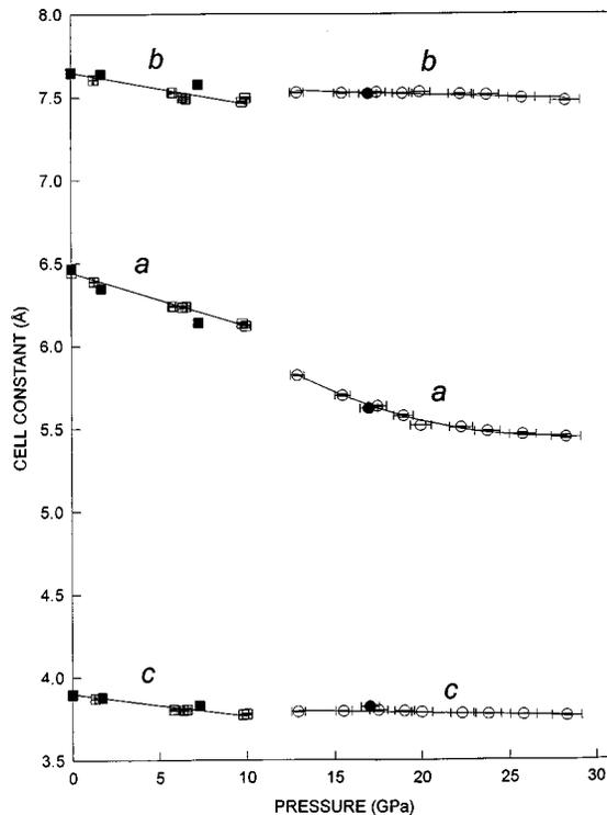
FIG. 1. Cell constants of  $\text{PbF}_2$  as a function of pressure. Open symbols refer to points obtained upon compression and solid symbols to those obtained upon decompression. Symbols  $\square$  and  $\circ$  correspond to  $\alpha$ - and  $\gamma$ - $\text{PbF}_2$ , respectively. Solid lines represent least squares fits to the data.
