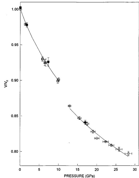
FIG. 2. Relative volume of  $\text{PbF}_2$  as a function of pressure. Legend as for Fig. 1. Solid lines represent Birch-Murnaghan equations of state using the parameters obtained in this study.
