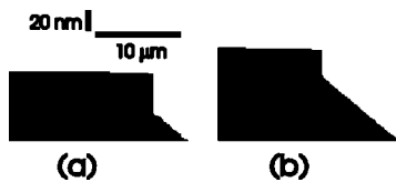
FIG. 10. Simulated sideplane cross sections with A_c=35 \mu\text{m}^2 shown at a larger scale for a=0.50 (a) and a=0.55 (b).
