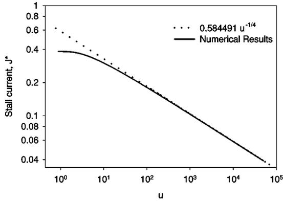
FIG. 6. A log-log plot of the stall current  $J^*$  vs  $u$ . The solid line shows the numerically determined  $J^*$ 's as a function of  $u$  and the dotted line is  $0.584491 u^{-1/4}$  (the large- $u$  behavior predicted by matched asymptotic analysis).
