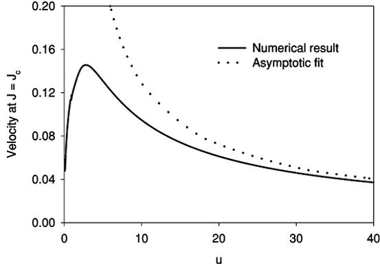
FIG. 10. The velocity as  $J \rightarrow J_c$  as a function of  $u$ . For large  $u$ , the velocity asymptotically approaches  $0.92u^{-0.85}$ .
