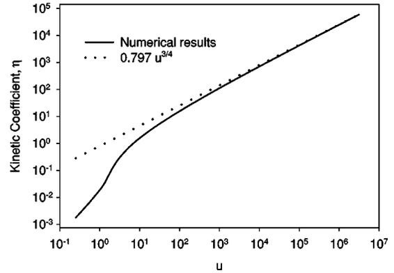
FIG. 8. A log-log plot of the numerically determined kinetic coefficient as a function of  $u$  (solid line) along with an asymptotic fit of  $0.797u^{3/4}$  (dotted line).
