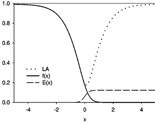
FIG. 4. The stationary NS interface solution when  $u=500$  for which the stall current  $J^*=0.12252$ . Shown here are the numerically determined  $f(x)$  and  $E(x)$ , as well as the Langer-Ambegaokar (LA) solution [Eq. (4.10), the solution with no electric field] corresponding to the same current.
