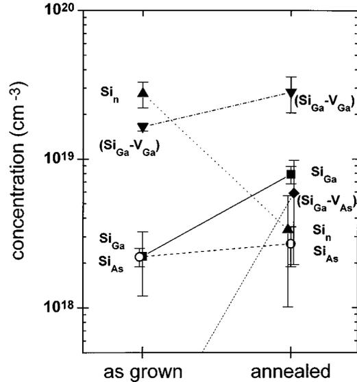
FIG. 2. Concentration of Si incorporated in different defects in the as-grown and in the annealed GaAs crystal. The lines connecting the points should guide the eye.  $\text{Si}_{\text{Ga}}$ ,  $\text{Si}_{\text{As}}$ ,  $(\text{Si}_{\text{Ga}}\text{-V}_{\text{Ga}})$ ,  $\text{Si}_n$ , and  $(\text{Si}_{\text{Ga}}\text{-V}_{\text{As}})$  refer to Si donors (■), Si acceptors (○), Si donor–Ga vacancy complexes (▼), Si pairs and clusters (▲), and Si donor–As vacancy complexes (◆), respectively.
