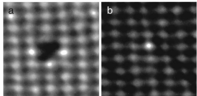
FIG. 1. Occupied (a) and empty (b) density of state images of the defect formed during tempering. The images have been acquired at  $-2.5$  and  $+2.2 \text{ V}$  ( $0.3 \text{ nA}$ ), respectively. The defect is a  $\text{Si}_{\text{Ga}}$  donor-As vacancy complex (see text).
