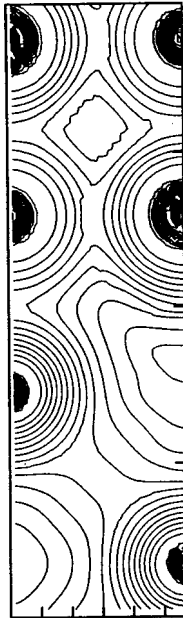
FIG. 11. Charge density contour of CdS/LaS for a section focused on the interface. The Cd atoms are the lowermost two atoms. In this figure there is a La atom in the top left corner of the figure. Below this La atom there is a S atom. There is also a S atom in the upper right corner of this figure that has a La atom just below it.
