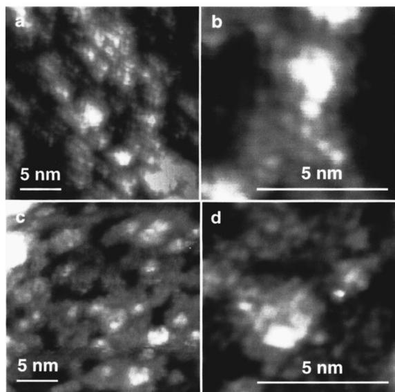
FIG. 1. STM images of the cleaved Al-Pd-Mn quasicrystal surfaces at room temperature. (a) and (b) show the cleavage surface perpendicular to a twofold direction at different magnifications, whereas (c) and (d) show the fivefold surface at two magnifications. The constant current images (1 nA current) were measured at tunneling voltages of  $-225$ ,  $-300$ ,  $-350$ , and  $-350$  mV, respectively.
