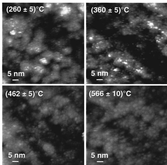
FIG. 4. Surface structure of the fivefold cleaved surface after heat treatment at  $(260 \pm 5)$ ,  $(360 \pm 5)$ ,  $(462 \pm 5)$ , and  $(566 \pm 10)$  °C. The scan area is  $70 \times 70$  nm<sup>2</sup>. The images were measured at tunneling voltages of  $-1.5$ ,  $-1.6$ ,  $+1.6$ , and  $+1.7$  V, respectively, (0.6 nA tunnel current). The corrugation is between 1.5 and 2.5 nm for all temperatures.
