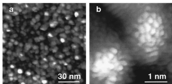
FIG. 5. (a) Cluster-based structure observed in a surface area maintaining its metallic reflectivity during annealing at  $(580 \pm 40)$  °C for 2.5 h. (b) High-resolution image of (a). (a) and (b) were measured at tunneling voltages of  $-1.1$  and  $-0.67$  V, respectively.
