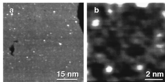
FIG. 6. (a) Flat terrace with a corrugation of less than 0.1 nm observed in an area affected by evaporation such as that in Fig. 3(b) during annealing at  $(550 \pm 10)$  °C for 2.5 h. (b) High-resolution image of the terrace structure [enhanced contrast compared to (a)]. The images were measured at a tunneling voltage of  $-1.5$  V.
