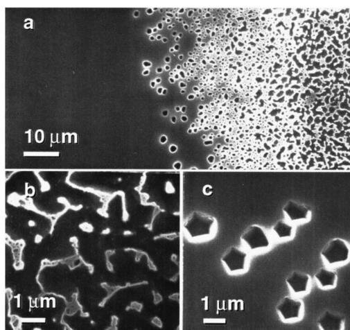
FIG. 3. (a) Scanning electron microscopy image of the cleaved and heat-treated fivefold icosahedral Al-Pd-Mn quasicrystal surface. In the left-hand part no modification occurred during heat treatment at  $550$  °C for 1 h, while in the right-hand part holes were formed by desorption. (b) Magnified area of a surface area with an almost full layer removed by desorption under the same conditions. (c) Faceted holes with a low density exhibiting a fivefold edge orientation.
