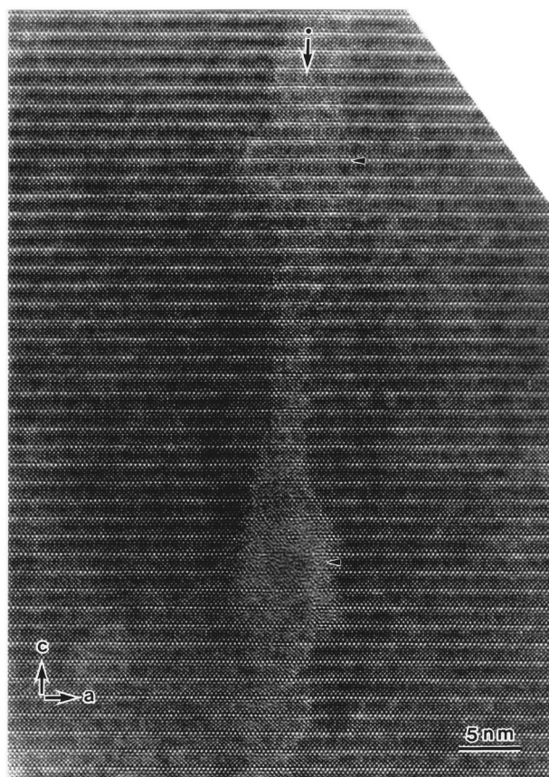
FIG. 4. HREM image showing the structural detail of the cascade-defect-dotted columnar defect. The black triangles indicate the positions of cascade defects and the arrow shows the ion penetration direction. The columnar defect can be seen clearly between two cascade defects.
