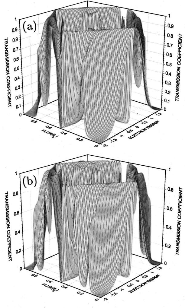
FIG. 7. Transmission coefficient  $T$  as a function of magnetic flux  $\Phi$  and incident electron energy  $E$  for serial multiring systems with (a) six rings and (b) eight rings. Note the complicated structures in the transmission coefficient due to the coupling among the rings.
