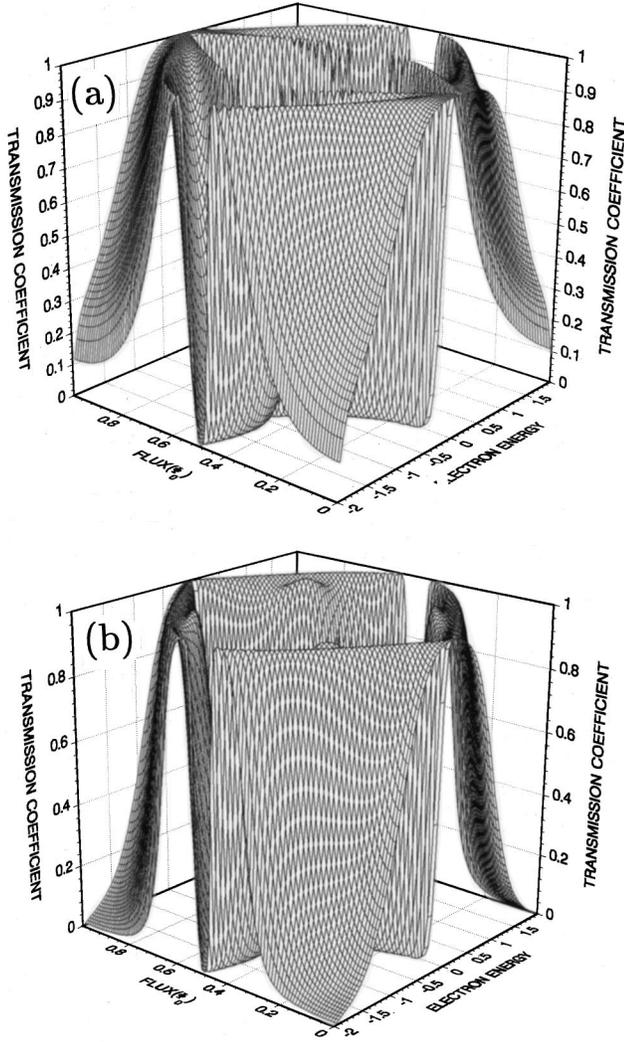
FIG. 6. Transmission coefficient  $T$  as a function of magnetic flux  $\Phi$  and incident electron energy  $E$  for serial multiring systems with (a) two rings and (b) four rings.
