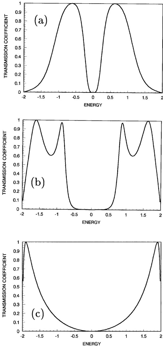
FIG. 8. Transmission coefficient  $T$  vs electron energy  $E$  for serial six-ring systems with (a) flux  $\Phi = 0.1\Phi_0$ , (b)  $\Phi = 0.3\Phi_0$ , and (c)  $\Phi = 0.4\Phi_0$ . The relationship between  $T$  and  $E$  is clearly shown.
