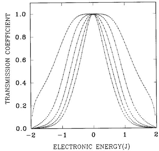
FIG. 9. Transmission coefficient  $T$  for serial multiring systems as a function of incident energy in the absence of magnetic flux, i.e.,  $\Phi = 0$ . The five curves from top to bottom correspond to systems with two rings, four rings, six rings, eight rings, and ten rings, respectively. Note that the transmission coefficient depends sensitively on the number of rings in SRS.
