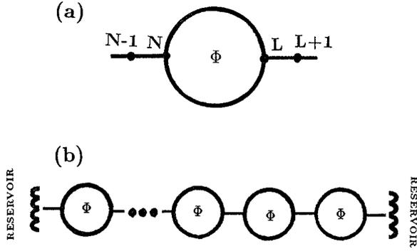
FIG. 1. (a) A single ring coupled to two reservoirs via two leads. (b) Multirings threaded by magnetic flux  $\Phi$ , connected in series, and coupled to two reservoirs via ideal leads.
