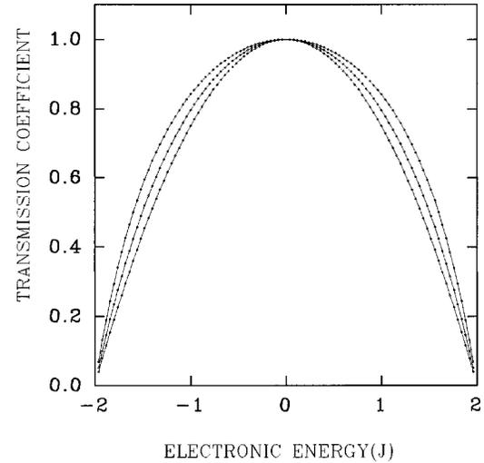
FIG. 5. Transmission coefficient  $T$  for parallel multiring systems as a function of incident energy in the absence of magnetic flux, i.e.,  $\Phi = 0$ . The three curves from top to bottom correspond to systems with 2 rings, 16 rings, and 1024 rings, respectively. The transmission coefficient decreases only slightly as the number of rings increases in PRS.
