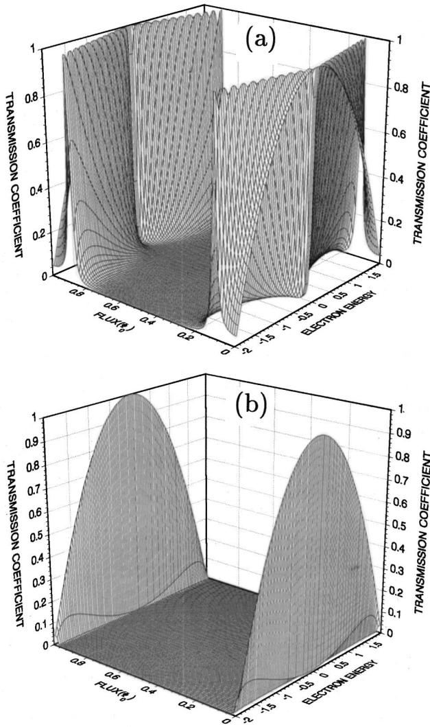
FIG. 4. Transmission coefficient  $T$  as a function of magnetic flux  $\Phi$  and incident electron energy  $E$  for parallel multiring systems with (a) 16 rings, and (b) 4096 rings. Note that the region in the  $E$ - $\Phi$  plane corresponding to vanishing transmission increases as the number of rings increases.
