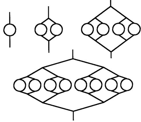
FIG. 2. Parallel multiring system in which only the rings are assumed to be threaded by a magnetic flux  $\Phi$ . All of the rings are assumed to be identical.
