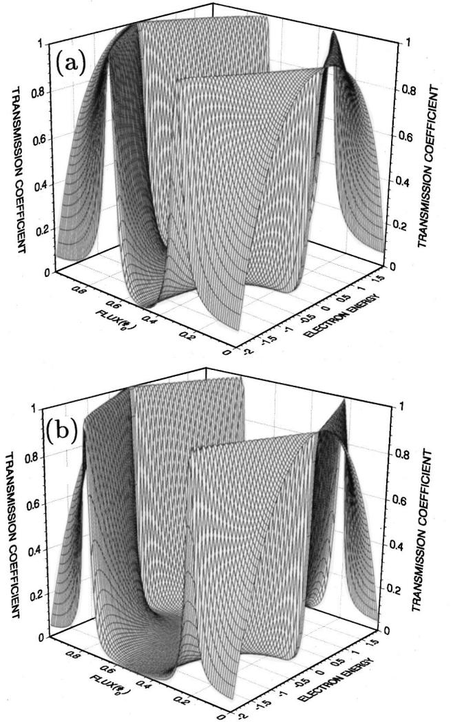
FIG. 3. Transmission coefficient  $T$  as a function of magnetic flux  $\Phi$  and incident electron energy  $E$  for parallel multiring systems with (a) two rings and (b) four rings.
