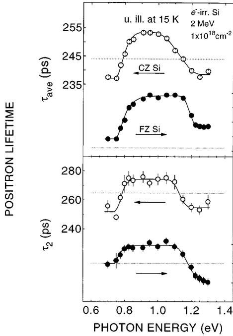
FIG. 2. Positron lifetime in electron-irradiated Si at 15 K under illumination with monochromatic light. The photon flux is  $1 \times 10^{16} \text{ cm}^{-2} \text{ s}^{-1}$ . The average positron lifetime  $\tau_{\text{ave}}$  and the long lifetime component  $\tau_2$  are presented as a function of the illumination photon energy: (●) FZ Si (sample F1) and (○) CZ Si (sample C2). The dotted lines show the positron lifetime in darkness at 15 K. The solid lines are guides to the eye.
