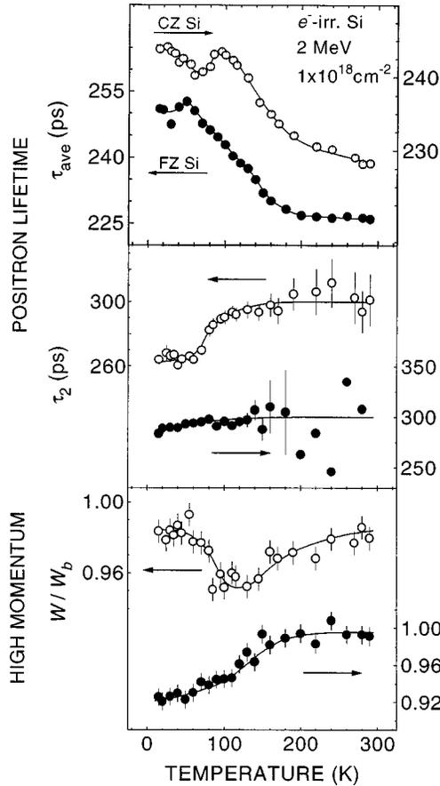
FIG. 1. Average positron lifetime  $\tau_{\text{ave}}$ , the second component  $\tau_2$  of the two-component lifetime spectrum, and the high-momentum parameter  $W$  of the Doppler-broadened annihilation line vs measurement temperature in electron-irradiated Si: (●) FZ Si (sample *F1*) and (○) CZ Si (sample *C2*). The solid lines are guides to the eye.
