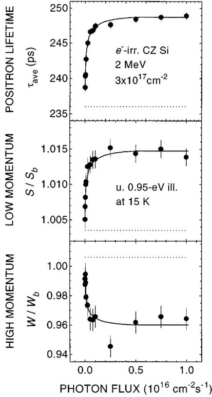
FIG. 4. Positron lifetime and Doppler broadening measured in the electron-irradiated CZ Si sample *C1* at 15 K under illumination with 0.95-eV light. The average positron lifetime  $\tau_{\text{ave}}$  and the  $S$  and  $W$  parameters are presented as a function of the illumination photon flux. The dotted lines show the values of  $\tau_{\text{ave}}$ ,  $S$ , and  $W$  measured in darkness at 15 K. The solid lines are guides to the eye.
