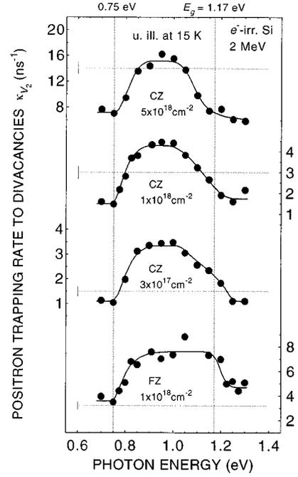
FIG. 8. Positron trapping rate  $\kappa_{V_2}$  to divacancies in electron-irradiated FZ Si (sample *F1*) and CZ Si (samples *C1*–*C3*) at 15 K under illumination with monochromatic light. The dotted horizontal lines indicate the values of  $\kappa_{V_2}$  in darkness at 15 K. The solid lines are guides to the eye.
