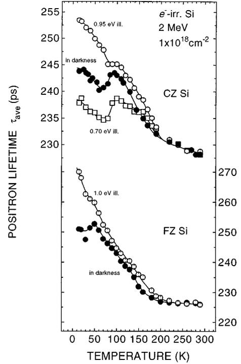
FIG. 5. Average positron lifetime  $\tau_{\text{ave}}$  in darkness and under illumination vs the measurement temperature in electron-irradiated Si. FZ Si sample *F1*, (●) in darkness and (○) under 1.0-eV illumination, CZ Si sample *C2*, (●) in darkness, (○) under 0.95-eV illumination, and (□) under 0.70-eV illumination. The solid lines are guides to the eye.
