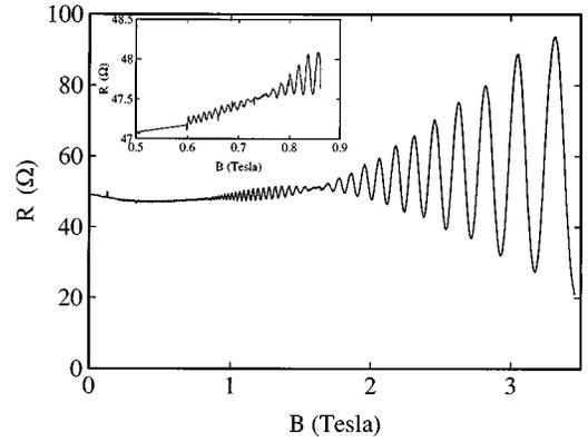
FIG. 2. Longitudinal magnetoresistance  $\rho_{xx}$  at  $T=1.3$  K and  $V_{\text{gate}}=1$  V. The inset shows the left beat at a different scale.
