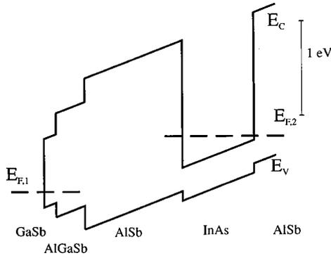
FIG. 1. Schematic AlSb/InAs/AlSb heterostructure band diagram with an applied positive gate voltage, ignoring band bending.  $E_{F,1}$  and  $E_{F,2}$  are the left and right Fermi energies, respectively.  $E_c$  is the conduction band, and  $E_v$  the valence band.
