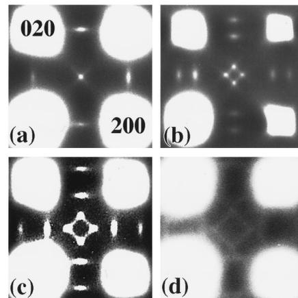
FIG. 1.  $[001]$  electron-diffraction patterns of  $\text{Cu}_{1-x}\text{Pd}_x$ , where  $x=0.10$  (a),  $0.30$  (b),  $0.40$  (c), and  $0.50$  (d). In (c), the contrast is overenhanced in order to visualize the diffuse streaks, perpendicular to the twofold splitting or connecting the spots in the fourfold splitting.
