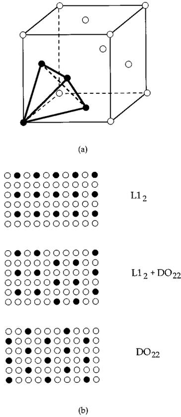
FIG. 2. (a) Tetrahedron (in bold) of nearest neighbors in an fcc cube. (b) Examples of stacking an  $A_3B$  structure so that Eq. (7) is fulfilled for all lattice sites. Only two nonoverlapping (001) layers have been drawn. Empty circles represent  $A$  atoms, filled circles,  $B$  atoms.
