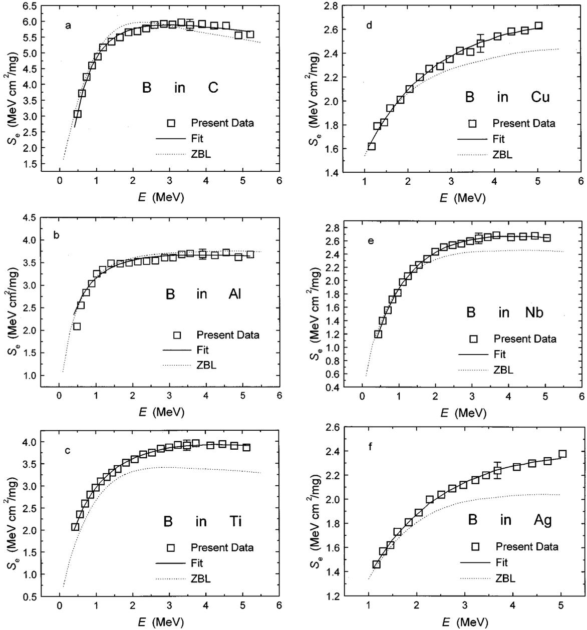
FIG. 1. Stopping power for  $^{11}\text{B}$  in C (a), Al (b), Ti (c), Cu (d), Nb (e), and Ag (f).
