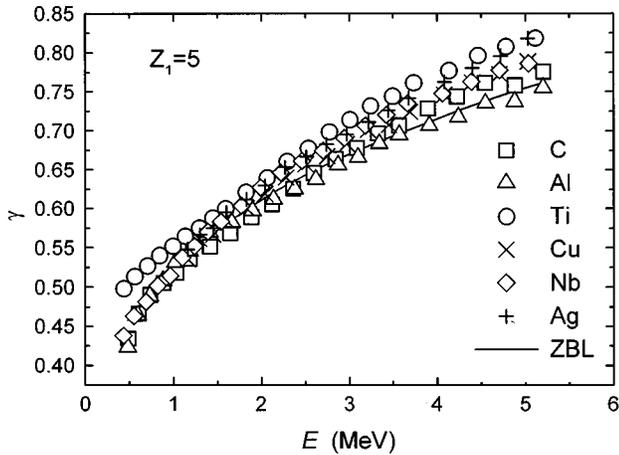
FIG. 2. Comparison of effective charge versus energy between present data and ZBL approaches.
