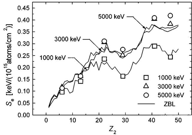
FIG. 3. Dependence of  $^{11}\text{B}$   $S_e$  on  $Z_2$ .
