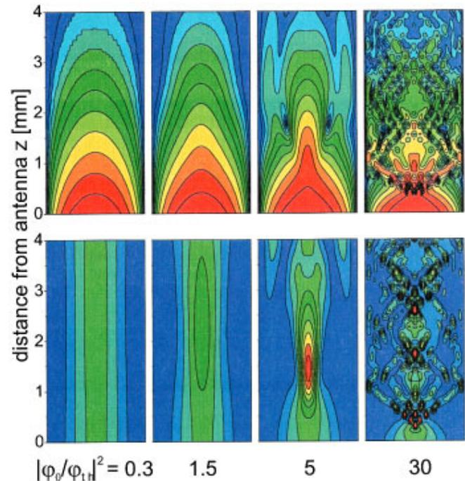
FIG. 3. (Color) Numerically calculated stationary distribution of the spin-wave intensity. Upper panels show  $|\varphi(y,z)|^2$  normalized to the maximum intensity  $|\varphi_0|^2$  of the initial ( $z=0$ ) beam intensity distribution in a logarithmic scale. Lower panels show  $|\varphi/\varphi_0|^2 \exp(\kappa z)$  in a linear scale.
