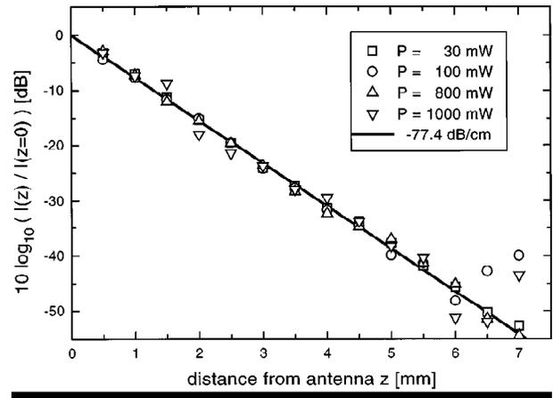
FIG. 2. Integrated intensity of the spin-wave modes  $I(z)$  as a function of the distance to the antenna normalized to its extrapolated value at  $z=0$ . The attenuation parameter obtained from a fit (full line) is  $\kappa = 77.4 \pm 1.5$  dB/cm.
