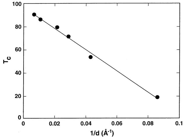
FIG. 2. Change in zero-resistance transition temperature,  $\Delta T_c = T_c^{\text{bulk}} - T_c(d)$ , of superconducting YBCO layers separated by 16 unit cells ( $\sim 187$  Å) of PrBCO, as a function of the reciprocal of the total YBCO layer thickness. The line is a linear fit to the data.
