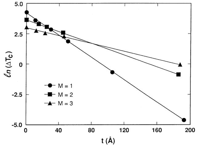
FIG. 3. Natural logarithm of  $\Delta T_c = T_c(d, t) - T_c(d, t = \infty)$  for YBCO layers with thicknesses corresponding to  $M = 1, 2$ , and 3  $c$ -axis unit cells as a function of PrBCO separation layer thickness. The lines are linear fits to the data.
