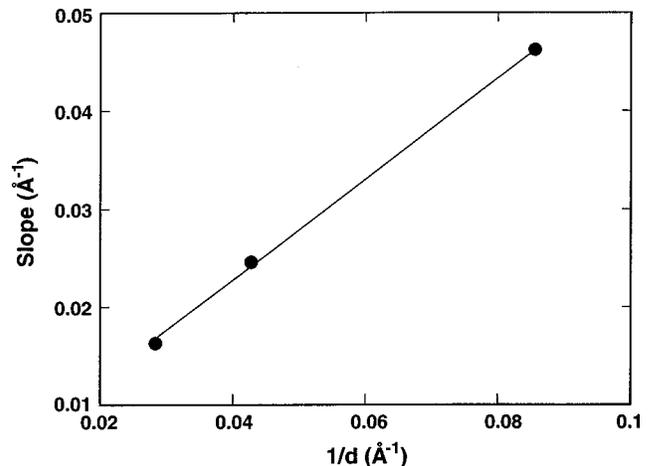
FIG. 4. Slopes of the linear fits in Fig. 3 as a function of the reciprocal of the distance between the superconducting layers. The line is a fit to the data.
