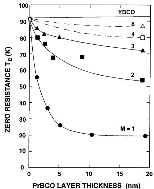
FIG. 1. Zero-resistance transition temperature as a function of PrBCO layer thickness for c-axis perpendicular YBCO/PrBCO superlattices with  $M=1, 2, 3, 4,$  and  $8$  cell-thick superconducting YBCO layers.
