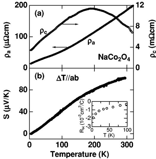
FIG. 2. (a) In-plane ( $\rho_a$ ) and out-of-plane ( $\rho_c$ ) resistivity of  $\text{NaCo}_2\text{O}_4$  single crystals. (b) In-plane thermoelectric power ( $S$ ) of  $\text{NaCo}_2\text{O}_4$  single crystal. The inset shows the in-plane Hall coefficient ( $R_H$ ) of  $\text{NaCo}_2\text{O}_4$  single crystal.
