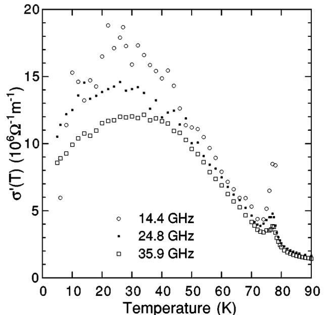
FIG. 4.  $\sigma'(T)$  at 14.4, 24.8, and 35.9 GHz displays a broad, frequency-dependent peak at low  $T$ .
