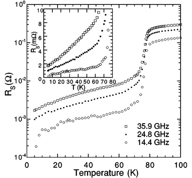
FIG. 1.  $R_s$  shows a sharp transition at 78 K and characteristic  $\omega^2$  frequency dependence at lower temperatures, indicating good homogeneity. Inset:  $R_s$  on a linear scale.
