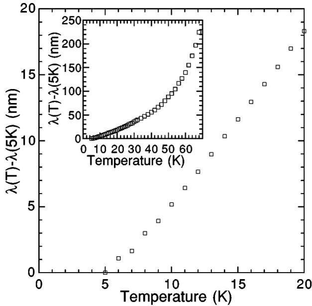
FIG. 2.  $\Delta\lambda(T) = \lambda(T) - \lambda(5 \text{ K})$  displays a strong linear term at low  $T$ . Inset:  $\Delta\lambda(T)$  over a wider temperature range.
