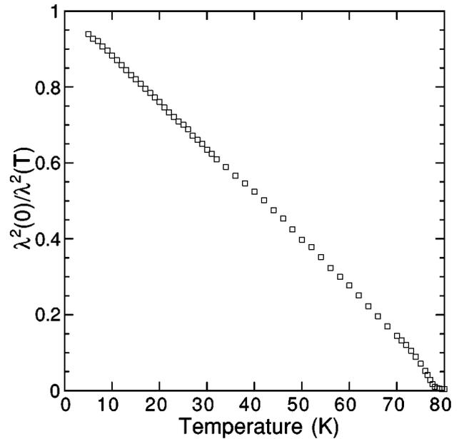
FIG. 3.  $f_s(T) = \lambda^2(0)/\lambda^2(T)$  (from  $\sigma''$ ) shows a linear temperature dependence over most of the superconducting state, with a rapid downturn near  $T_c$ .
