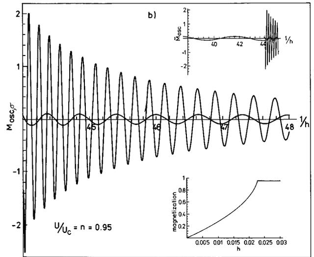
FIG. 4. The shape of the oscillatory component of magnetization vs  $1/h$  in the Fermi-liquid regime (a), and near the ALFL  $\rightarrow$  SSL transition. (b) The upper inset illustrates the evolution of the de Haas–van Alphen oscillations across the metamagnetic transition whereas the lower specifies the shape of the magnetization curve in this case.
