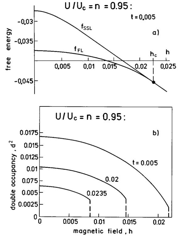
FIG. 1. (a) Field dependence of the free energies for an almost localized Fermi liquid  $f_{FL}$  and for the correlated liquid ( $f_{SSL}$ ). The ALFL is unstable for  $h > h_c$ ; (b) the variation of the double occupancy probability.
