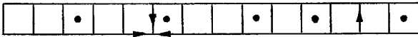
FIG. 5. If the stack of shifted 1D vortex lattices is to leave the phase configuration intact, as energy is minimized in the quenching process, each site must be in its local minimum before quenching. Therefore currents into each site of the complete vortex lattice must sum to zero, to begin with. This implies that the generator should obey Eq. (6). Here, the currents that participate in that equation are indicated for one of the sites. Compare with Fig. 3.
