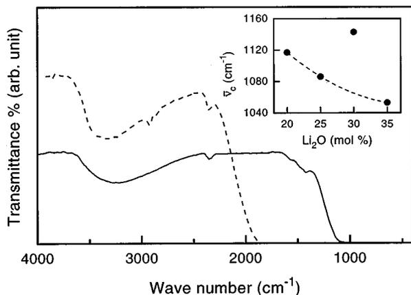
FIG. 6. FTIR spectra of  $30\text{Li}_2\text{O}-70\text{Bi}_2\text{O}_3$  (solid curve) and  $\text{PbO}-\text{Bi}_2\text{O}_3$  (dashed curve) glasses. Inset shows the variation of  $\bar{\nu}_c$  with the  $\text{Li}_2\text{O}$  content in the lithium bismuthate glasses.
