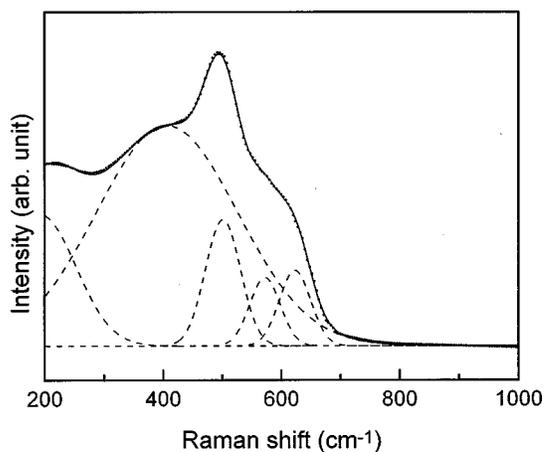
FIG. 7. Raman spectrum of  $30\text{Li}_2\text{O}-70\text{Bi}_2\text{O}_3$  glass composition. Deconvoluted peaks are indicated by dashed curves.
