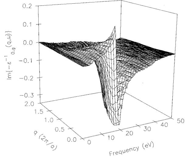
FIG. 1. The higher-order loss function  $\text{Im}\{-\varepsilon_{0,\mathbf{G}}^{-1}(|\mathbf{q}|,\omega)\}$ ,  $\mathbf{G} = (2\pi/a)(1,1,1)$  for silicon as a function of wave vector and frequency.
