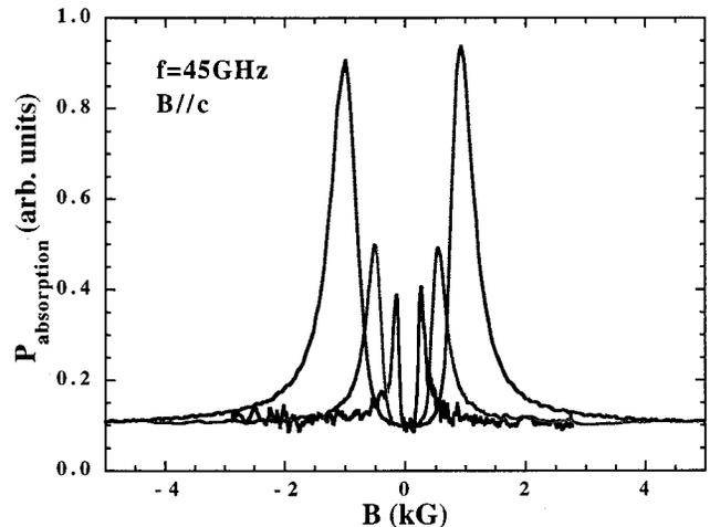
FIG. 2. A typical example of the microwave absorption spectrum at 45 GHz in a cavity shown in Fig. 1 in a perpendicular magnetic field ( $\mathbf{B} \parallel c$ ) at three different temperatures. The resonances observed are plotted at 22.5 K (outer curve), 44.9 K (middle curve), and 66.9 K (inner curve). The vertical scale is taken arbitrarily but the relative intensity is kept unchanged.
