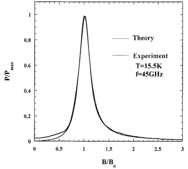
FIG. 5. The direct comparison of the absorption curve obtained from the experiments (thicker curve) with the calculated microwave power absorption spectrum (thinner curve) at 45 GHz as a function of  $B$  applied along the  $c$  axis using Eq. (5). The values of  $\mu = 15$  Å and  $L = 20$  μm are used for numerical calculations.
