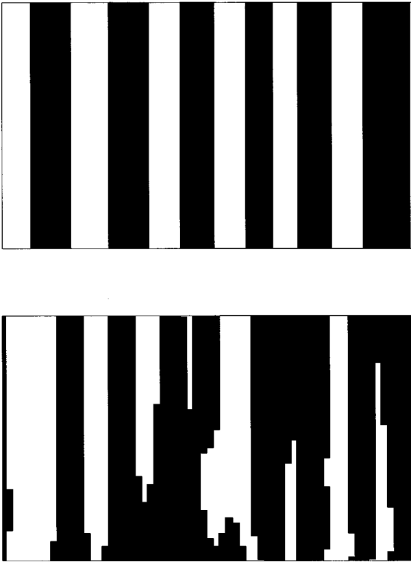
FIG. 3. A vertical cross section of the thin film taken along the x direction. The bottom configuration shows the appearance of the thin film at early times ( 0 < \tau < 100 ), while the top configuration corresponds to the steady state ( 1400 < \tau < 1500 ). The lateral size of the system is 128 and the vertical scale is chosen to show details.
