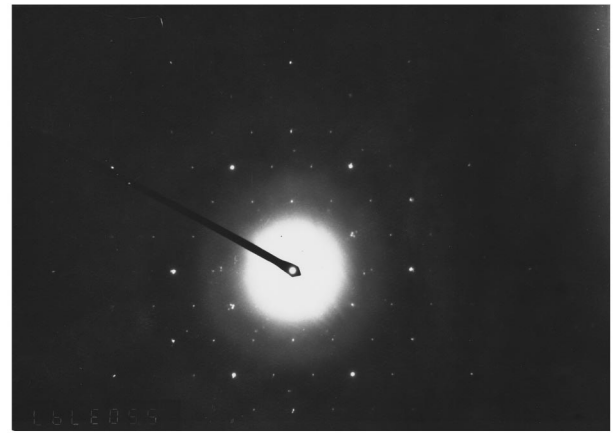
FIG. 3. The transmission electron diffraction pattern of a \text{C}_3\text{N}_4 film deposited on \text{Si}_3\text{N}_4 . The sample was annealed at 800^\circ\text{C} in vacuum for 2 h before TED measurement.
